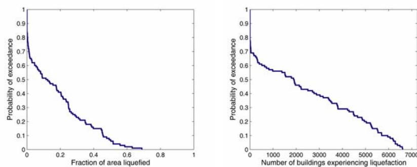
$$P(Y > y | pga, m) = \int_{\eta} I(h(g(\eta | pga, m) > y)) f_{\eta}(e) de$$
