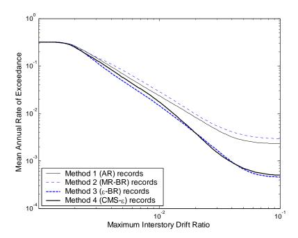
Figure 6.13: Mean annual frequency of exceeding various levels of maximum interstory drift ratio, as computed using the scalar intensity measure  $Sa(T_1)$ .
