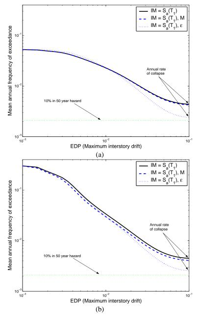
Figure 3.7. Seven story reinforced concrete frame. Mean annual frequency of exceedance versus maximum interstory drift. (a) Scalar-based and vector-based drift hazard curves for the Characteristic Event hazard; and (b) Scalar-based and vector-based drift hazard curves for the Van Nuys hazard.
