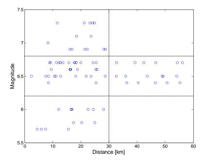
Figure A.1. Magnitudes and distances of the primary and secondary datasets (Table A.1 and Table A.2) used for analysis of the Van Nuys Testbed building.
