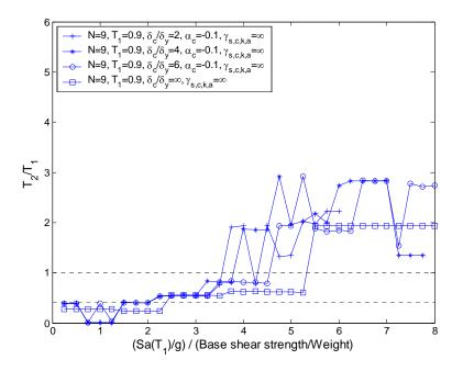
Figure 4.13: The optimal  $T_2$ , normalized by first-mode period  $(T_1)$  for a set of nine-structures with varying levels of element ductility.
