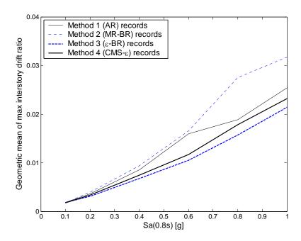
Figure 6.9: The geometric mean of maximum interstory drift ratio for records that do not cause collapse, plotted versus  $Sa(T_1)$  for the four record-selection methods considered. The x axis of the figure is truncated at 1g, because at higher levels of spectral acceleration, a significant fraction of records cause collapse.
