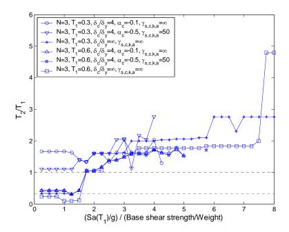
Figure 4.10: The optimal  $T_2$ , normalized by first-mode period  $(T_1)$  for a set of three-story structures dominated by first-mode response.
