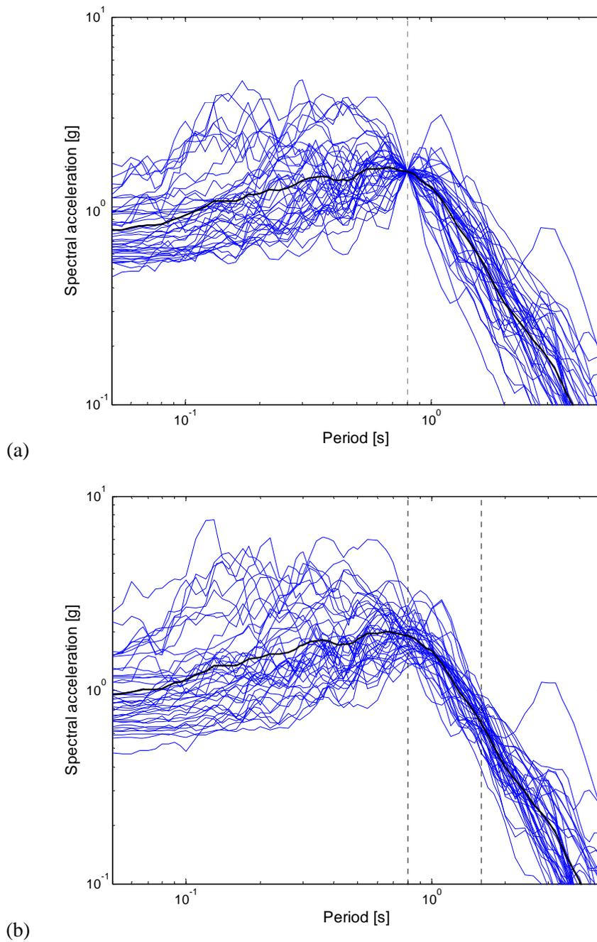
Figure 6.20: Records scaled to target 2% in 50 year IM levels. (a) Records scaled to  $\ln Sa(0.8s)$ . (b) Records scaled to  $\ln Sa_{avg}(0.8s, 1.6s)$ .
