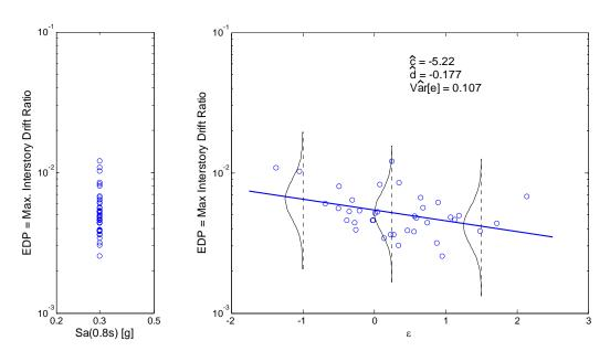
Figure 2.13. Prediction of response given no collapse, at Sa(0.8s) = 0.3g, with the distribution of the residuals superimposed over the data.
