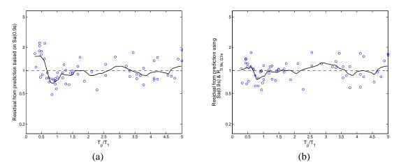
Figure 5.19. Residuals from response prediction based (a)  $Sa(T_1)$  only, and (b) both  $Sa(T_1)$  and  $R_{T_1,T_2}$ , plotted versus  $T_p/T_1$  for the generic frame with 9 stories and a first-mode period of 0.9 seconds, at an  $R_u$  factor level of 2.  $T_2 = 0.3$ s for this plot.
