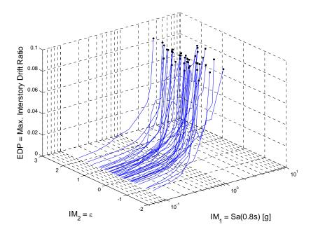
Figure 2.16. Incremental Dynamic Analysis with two intensity parameters, used to determine capacity in terms of the intensity measure.
