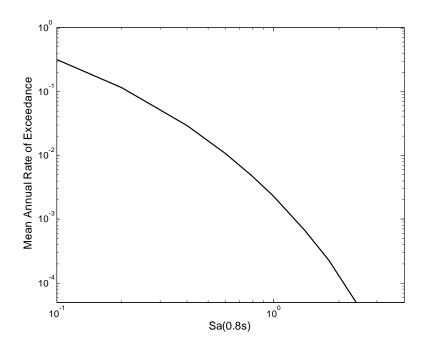
Figure 6.12: Mean annual frequency of exceeding various levels of Sa(0.8s) (i.e., the ground motion hazard curve), for the Van Nuys, California, site of interest.
