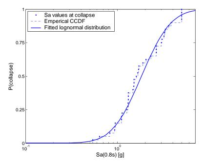
Figure D.2: Probability of collapse using an empirical CCDF and a fitted lognormal CCDF, for a set of records.
