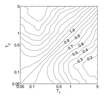
Figure B.1: Empirical spectral acceleration correlation contours for single ground motion components at two periods.
