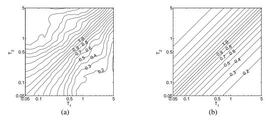
Figure 8.5. Correlation contours for vertical epsilons in the same direction at two periods (T1 and  $T_2$ ). (a) Smoothed empirical results. (b) The prediction from Equation 8.10.
