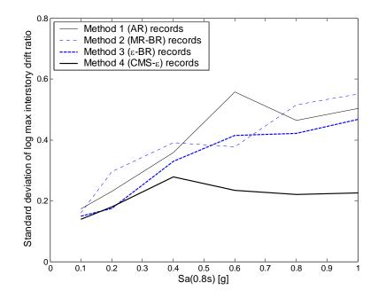
Figure 6.10: The standard deviation of log maximum interstory drift ratio for records that do not cause collapse, plotted versus  $Sa(T_1)$  for the four record-selection methods considered.
