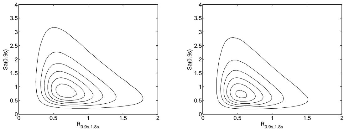
Figure 5.22. Joint conditional probability density function of  $Sa(T_1)$  and  $R_{T_1, T_2}$ , given a Magnitude 7 event at a distance of 5km, with the near-fault parameters  $X=0.5$  and  $\theta=5\%$ .  $T_1=0.9s$  and  $T_2=1.8s$ , in the fault-normal direction. (a) With near-fault effects considered. (b) Without near-fault effects considered.
