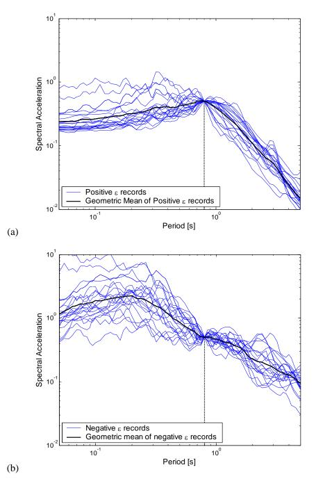
Figure 6.1: (a) Response spectra of records with the 20 largest  $\varepsilon$  values at 0.8s, and the geometric mean of the set, after scaling all records to Sa(0.8s)=0.5g. (b) Response spectra of records with the 20 smallest  $\varepsilon$  values at 0.8s, and the geometric mean of the set, after scaling all records to Sa(0.8s)=0.5g.
