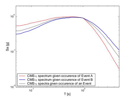
Figure E.5: Conditional mean spectra given occurrence of the individual events, and then combined CMS- $\varepsilon$  spectrum that is proposed as a target spectrum for record selection.
