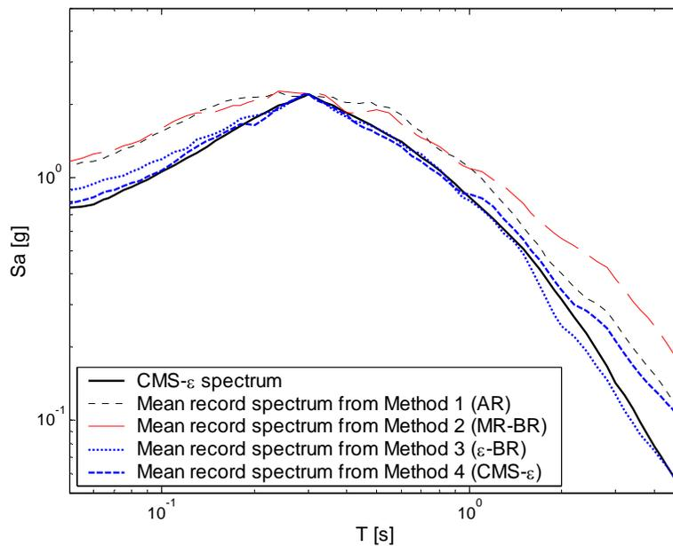
Figure F.1: Conditional Mean Spectra at  $Sa(0.3s)=2.2g$  (given  $\bar{M}=6.1$ ,  $\bar{R}=10.7$  km and  $\bar{\varepsilon}=2.1$ ) and the mean response spectra of record sets selected using each of the four proposed record selection methods.
