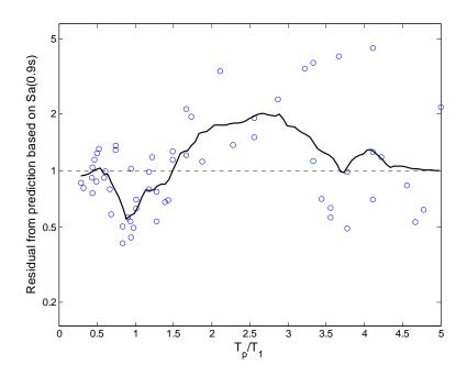
Figure 5.9. Residuals from response prediction based on  $Sa(T_1)$  plotted versus  $T_p/T_1$  for the generic frame with 9 stories and a first-mode period of 0.9 seconds, at an  $R_{\mu}$  factor level of 4.
