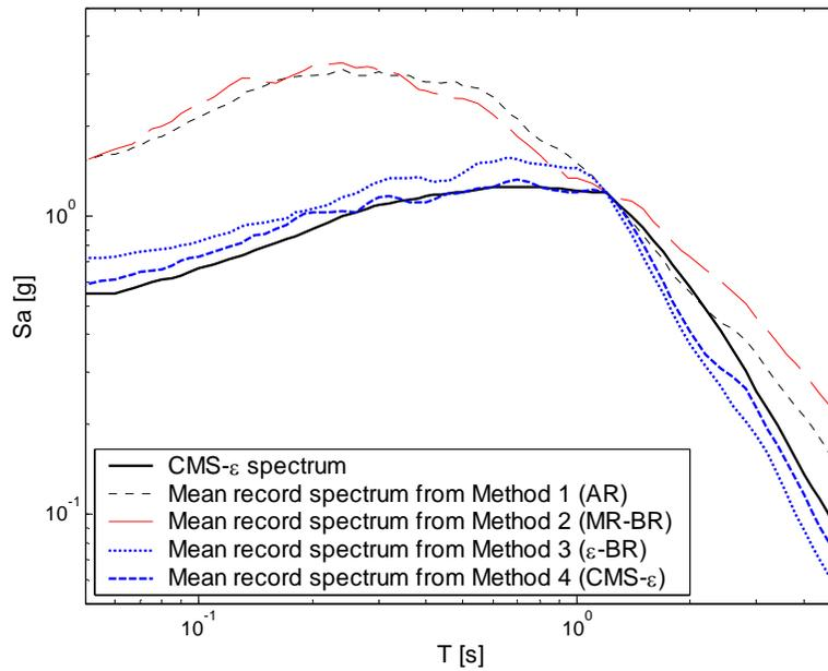
Figure F.7: Conditional Mean Spectrum at  $Sa(1.2s)=1.2g$  (given  $\bar{M}=6.6$ ,  $\bar{R}=15.8$  km and  $\bar{\varepsilon}=2.1$ ) and the mean response spectra of record sets selected using each of the four proposed record selection methods.
