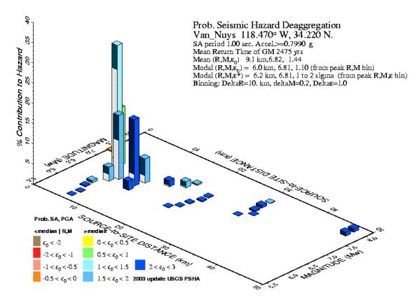
Lul 23 15:42 Distance (R), magnitude (M), epsilon (E0,E) desgregation for a site on ROCK avg Vs=760 mms top 30 m USGS CGHT PSHA2002x3 UPDATE Bins with th 0.05% contrib. omitted
