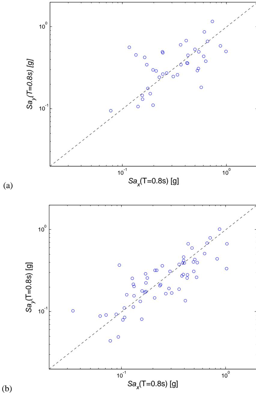
Figure 7.5. Samples of  $(\ln Sa_x, \ln Sa_y)$  pairs from (a) a set of ground motions with magnitude  $\approx 6.5$  and distance  $\approx 8\text{km}$ , and (b) a set of ground motions with a wider range of magnitudes and distances, used to perform the structural analyses displayed in Figure 7.3.
