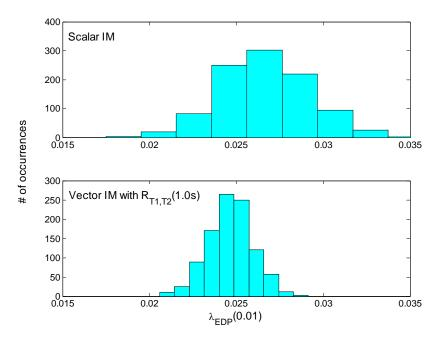
Figure 4.16: Histograms of the scalar and vector drift hazard curves, for z = 0.01.
