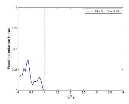
Figure 5.20. Percent reduction in the proposed bias statistic versus the  $T_2$  value used in  $R_{T1,T2}$ . Results are shown for the N=9,  $T_1 = 0.9$ s structure with an  $R_{\mu}$  factor of 2.
