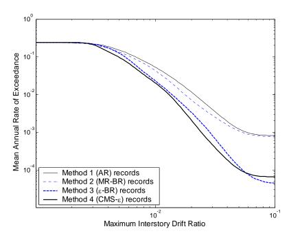
Figure F.11: Mean annual frequency of exceeding various levels of maximum interstory drift ratio, as computed using the *scalar* intensity measure  $Sa(T_1)$ .
