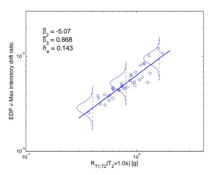
Figure 4.4: An example of non-collapse data, and a fit to the data using linear regression. The data comes from records scaled to  $S_a(T_1) = 0.3g$ . The estimated distributions of the residuals has been superimposed over the data.
