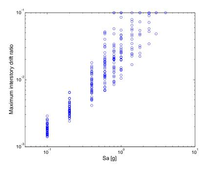
Figure 6.8: Maximum interstory drift ratio vs. Sa(0.8s). The results are shown for records from the Arbitrary Records method (i.e., Method 1). Similar results were obtained for the other three methods. Collapses are plotted as  $10^{-1}$  maximum interstory drift ratio, and the fraction of records causing collapse are indicated in Figure 6.11.
