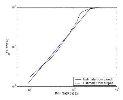
Figure 2.6. Mean values of *EDP*|*IM* for non-collapsing records, estimated using the cloud and stripe methods. For the stripe method, the values between stripes are determined using linear interpolation.
