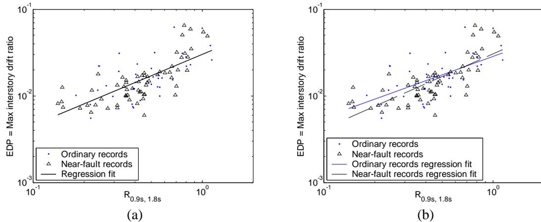
Figure 5.13. Prediction of response as a function of  $R_{0.9s, 1.8s}$  using linear regression on records scaled to an  $Sa(T_1)$  level such that the structure's  $R_\mu$  factor is 4. (a) Estimate of ordinary and pulse-like ground motion responses using the same prediction equation. (b) Estimate of ordinary and pulse-like ground motion responses using separate prediction equations.
