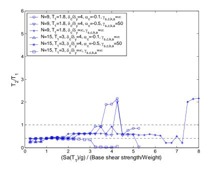
Figure 4.12: The optimal  $T_2$ , normalized by first-mode period ( $T_1$ ) for a set of nine- and fifteen-story structures with significant contribution from second-mode response.
