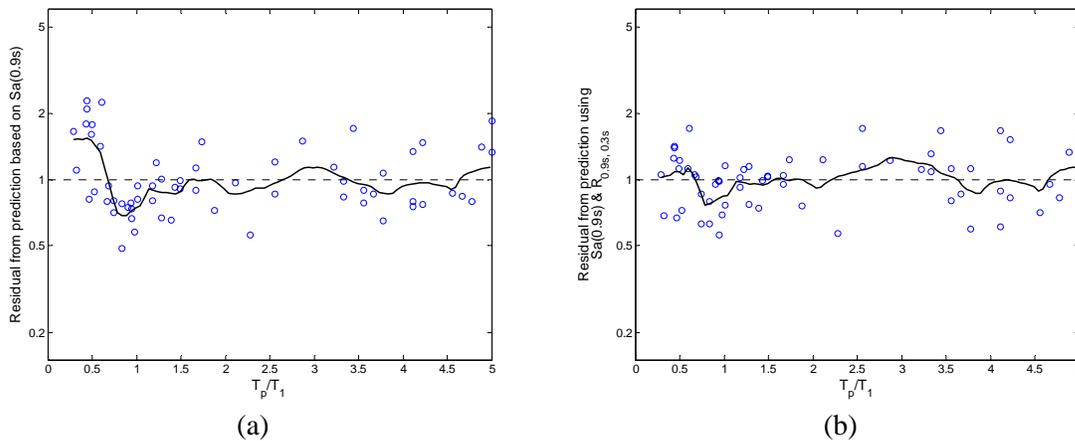
Figure 5.19. Residuals from response prediction based (a)  $Sa(T_1)$  only, and (b) both  $Sa(T_1)$  and  $R_{T_1,T_2}$ , plotted versus  $T_p/T_1$  for the generic frame with 9 stories and a first-mode period of 0.9 seconds, at an  $R_\mu$  factor level of 2.  $T_2=0.3s$  for this plot.
