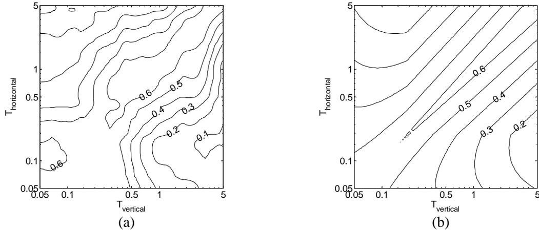
Figure 8.7. Correlation contours of vertical epsilons with horizontal epsilons at two periods ( $T_1$  and  $T_2$ ). (a) Smoothed empirical results. (b) The prediction from Equation 8.12.
