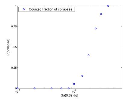
Figure D.3: Empirical probability of collapse for a set of *Sa* values, obtained from records selected to match target epsilon values at each *Sa* level.
