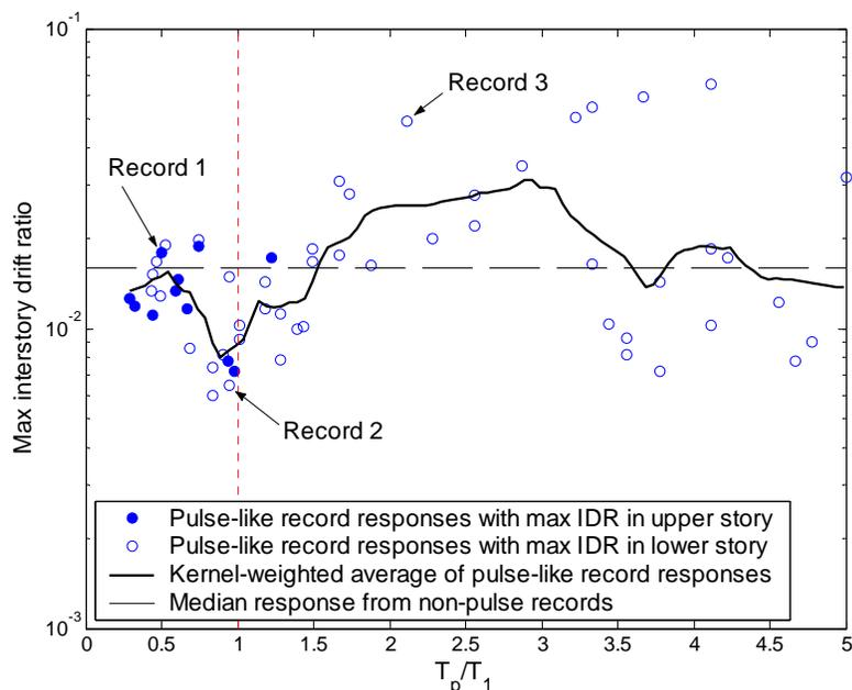
Figure 5.2. Maximum interstory drift ratio versus  $T_p/T_1$  for the generic frame with 9 stories and a first-mode period of 0.9 seconds, at an  $R_\mu$ -factor level of 4. Record 1: Morgan Hill, Anderson Dam (Magnitude = 6.2, Distance = 3km). Record 2: Kobe, KJMA (Magnitude = 6.9, Distance = 1km). Record 3: Superstition Hills, Parachute Test Site (Magnitude = 6.5, Distance = 1 km).
