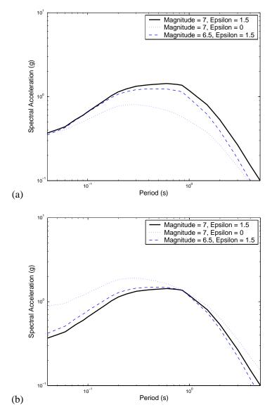
Figure 3.5. (a) Expected response spectra for three scenario events; (b) expected response spectra for three scenario events, scaled to have the same  $S_a(0.8s)$  value.
