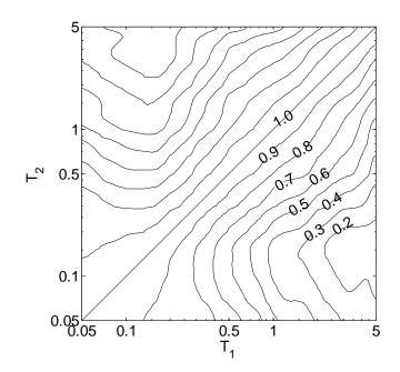
Figure B.2: Empirical spectral acceleration correlation contours for geometric means at two periods.
