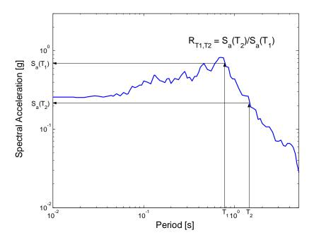
Figure 4.1: Illustration of the calculation of  $R_{T1,T2}$  for a given response spectrum.
