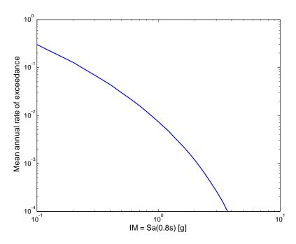
Figure 2.8. Ground motion hazard at the Van Nuys, California site for spectral acceleration at 0.8 seconds.
