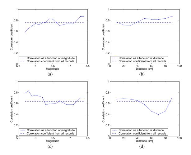
Figure B.7: Correlation coefficients for  $\varepsilon$  values at a period of 1 second as a function of magnitude and distance. (a) Opposite horizontal components versus magnitude. (b) Opposite horizontal components versus distance. (c) Horizontal/vertical components versus magnitude. (d) Horizontal/vertical components versus distance.
