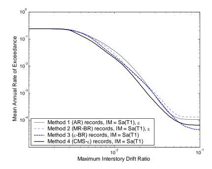
Figure F.12: Mean annual frequency of exceeding various levels of maximum interstory drift ratio, as computing using either the scalar intensity measure  $Sa(T_1)$  or the vector intensity measure  $Sa(T_1)$  and  $\varepsilon$ .
