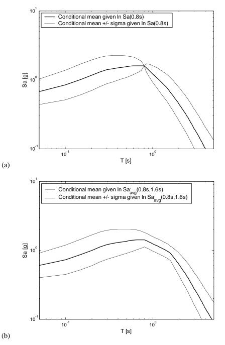
Figure 6.19: Conditional Mean Spectrum, considering  $\varepsilon$ , and +/ one standard deviation at the 2% in 50 year hazard level given (a)  $\ln Sa(0.8s)$ , and (b)  $\ln Sa_{avg}(0.8s, 1.6s)$ .
