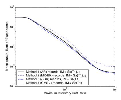
Figure 6.14: Mean annual frequency of exceeding various levels of maximum interstory drift ratio, as computing using either the scalar intensity measure  $Sa(T_1)$  or the vector intensity measure  $Sa(T_1)$  and  $\varepsilon$ .
