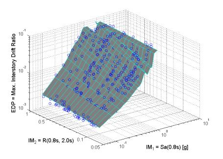
Figure 2.15. Conditional mean fit of non-collapse responses from stripes of data, predicted by scaling records to Sa(0.8s) and using repeated regressions with R(0.8s, 2.0s) as the predictor. In this case, the predicted mean is not planar, so it would be difficult to capture the true behavior using a cloud regression.
