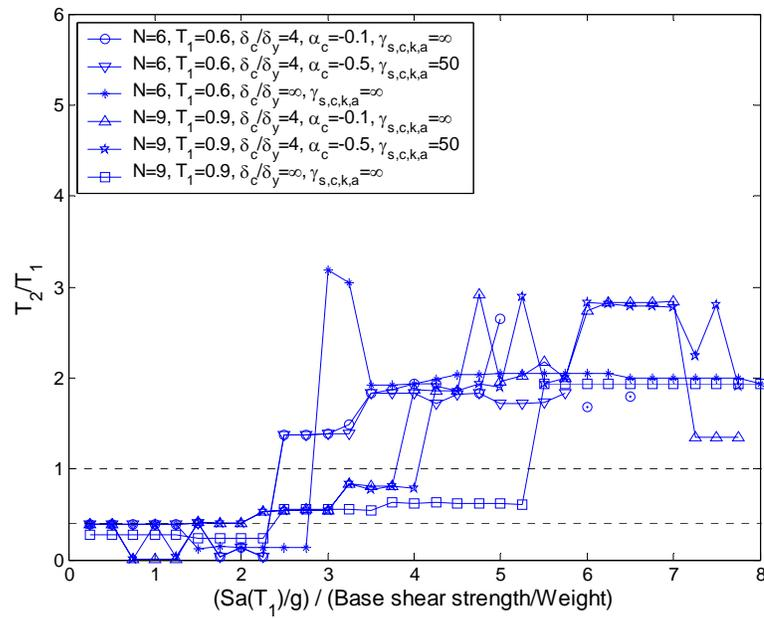
Figure 4.11: The optimal  $T_2$ , normalized by first-mode period ( $T_1$ ) for a set of six- and nine-story structures with moderate contribution from second-mode response.
