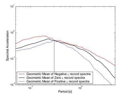
Figure 6.3: The geometric mean of response spectra for negative- $\varepsilon$ , zero- $\varepsilon$  and positive- $\varepsilon$  record sets, after each record's spectrum has been scaled to Sa(0.3s)=0.5g.
