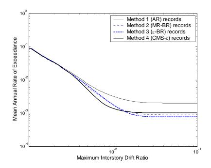
Figure F.5: Mean annual frequency of exceeding various levels of maximum interstory drift ratio, as computed using the *scalar* intensity measure  $Sa(T_1)$ .
