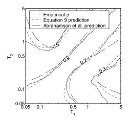
Figure 8.9. Overlaid contours at four correlation levels for the empirical correlations, the prediction from Equation 8.9 and the prediction from Abrahamson et al. (2003).
