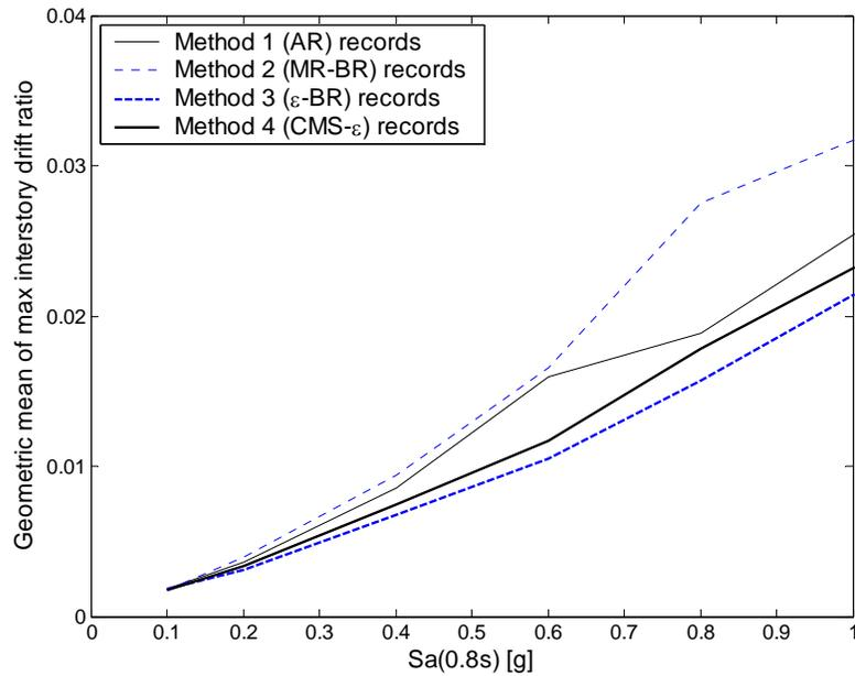
Figure 6.9: The geometric mean of maximum interstory drift ratio for records that do not cause collapse, plotted versus  $Sa(T_1)$  for the four record-selection methods considered. The x axis of the figure is truncated at 1g, because at higher levels of spectral acceleration, a significant fraction of records cause collapse.
