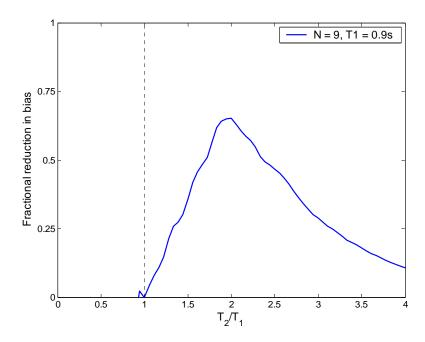
Figure 5.17. Percent reduction in the proposed bias statistic versus the  $T_2$  value used in  $R_{T1,T2}$ . Results are shown for the N=9,  $T_1 = 0.9$ s structure with an R<sub>µ</sub> factor of 4.
