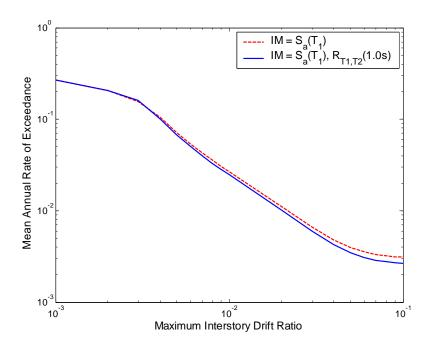
Figure 4.14: Maximum interstory drift hazard curves computed using a scalar IM and a vector IM
