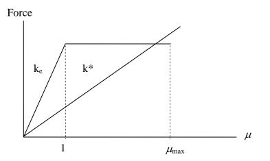
Figure 4.9: Schematic illustration of a non-linear SDOF and a potential equivalent linear system based upon maximum observed ductility.
