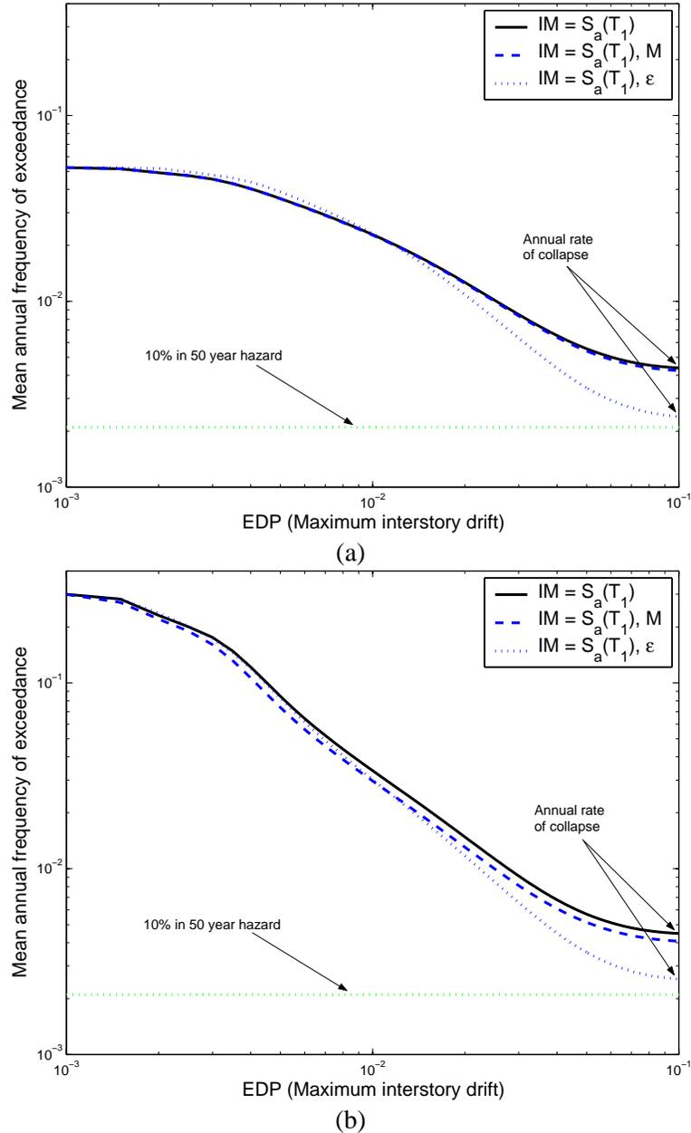
Figure 3.7. Seven story reinforced concrete frame. Mean annual frequency of exceedance versus maximum interstory drift. (a) Scalar-based and vector-based drift hazard curves for the Characteristic Event hazard; and (b) Scalar-based and vector-based drift hazard curves for the Van Nuys hazard.
