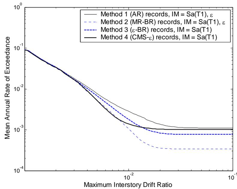
Figure F.6: Mean annual frequency of exceeding various levels of maximum interstory drift ratio, as computing using either the scalar intensity measure  $Sa(T_1)$  or the vector intensity measure  $Sa(T_1)$  and  $\varepsilon$ .
