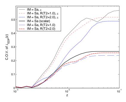
Figure 4.20: Coefficient of variation vs. *EDP* level for six candidate *Ims* consisting of one, two or three parameters.
