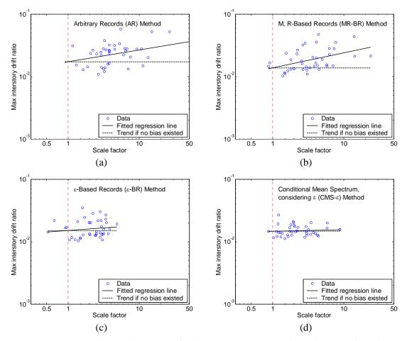
Figure F.13: Maximum interstory drift ratio versus record scale factor for each of the four selection methods considered, at an Sa(1.2s) level of 0.6g. Regression fits based on scale factor are shown with solid lines. Dashed horizontal lines corresponding to the mean prediction at a scale factor of one are shown for comparison. (a) Records using the AR Method. (b) Records using the MR-BR Method. (c) Records using the  $\varepsilon$ -BR Method. (d) Records using the CMS- $\varepsilon$  Method.
