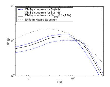
Figure 6.18: CMS- $\varepsilon$  spectra for  $\ln Sa(0.8s)$ ,  $\ln Sa(1.6s)$ , and  $\ln Sa_{avg}(0.8s, 1.6s)$  at the 2% in 50 year hazard level, and the 2% in 50 year uniform hazard spectrum.
