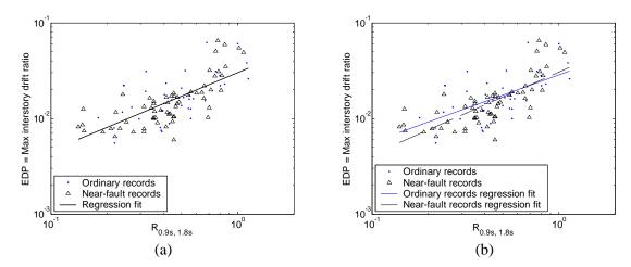
Figure 5.13. Prediction of response as a function of  $R_{0.9s,1.8s}$  using linear regression on records scaled to an  $Sa(T_1)$  level such that the structure's  $R_{\mu}$  factor is 4. (a) Estimate of ordinary and pulse-like ground motion responses using the same prediction equation. (b) Estimate of ordinary and pulse-like ground motion responses using separate prediction equations.
