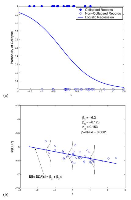
Figure 3.1. Analysis of data at a fixed value of  $S_a$ , (a) Prediction of the probability of collapse using logistic regression applied to binary collapse/non-collapse results; and (b) prediction of response given no collapse, with the distribution of the residuals superimposed over the data.
