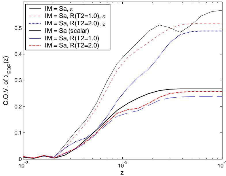
Figure 4.20: Coefficient of variation vs.  $EDP$  level for six candidate  $IMs$  consisting of one, two or three parameters.
