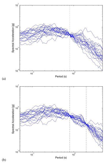
Figure 2.19. (a) Response spectra of records scaled to match spectral acceleration at a 0.8s. (b) Response spectra of records scaled to match spectral acceleration at 0.8s and processed to match spectral acceleration at 2.0s.
