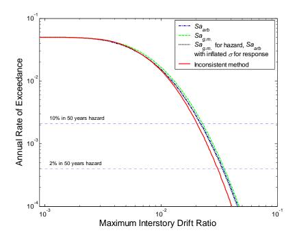
Figure 7.4. Drift hazard as computed using the three methods proposed above and the inconsistent method.
