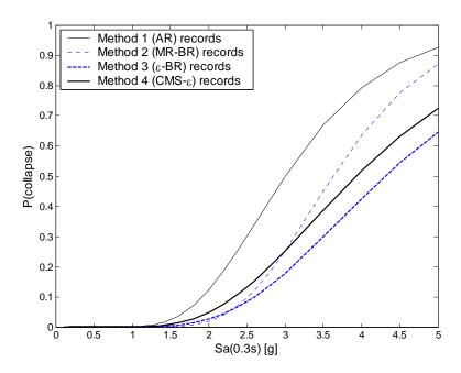
Figure F.4: Estimated probability of collapse vs.  $Sa(T_1)$  (i.e., the collapse "fragility curve") using the four record-selection methods considered.
