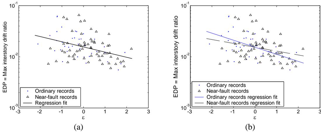
Figure 5.8. Prediction of response as a function of  $\varepsilon$  using linear regression on records scaled to have an  $R_{\mu}$  factor level of 4. (a) Estimate of ordinary and pulse-like ground motion responses using the same prediction equation. (b) Estimate of ordinary and pulse-like ground motion responses using separate prediction equations.
