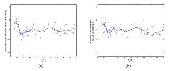
Figure 5.12. Residuals from response prediction based on (a)  $Sa(T_1)$  and (b)  $Sa(T_1)$  and  $\varepsilon$  plotted versus  $T_p/T_1$  for the generic frame with 9 stories and a first-mode period of 0.9 seconds, at an R<sub>µ</sub> level of 2. No significant reduction in bias is seen when  $\varepsilon$  is incorporated in the intensity measure.
