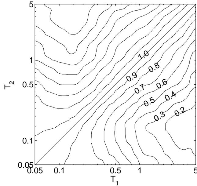
Figure B.1: Empirical spectral acceleration correlation contours for single ground motion components at two periods.
