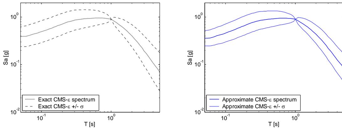
Figure E.7: (a) Exact conditional mean and standard deviation of the response spectrum, given  $Sa(1s)=0.9g$ . (using Equations E.2 and E.3). (b) Approximate conditional mean and standard deviation of the response spectrum, given  $Sa(1s)=0.9g$ . (using Equations 6.1 and 6.2).
