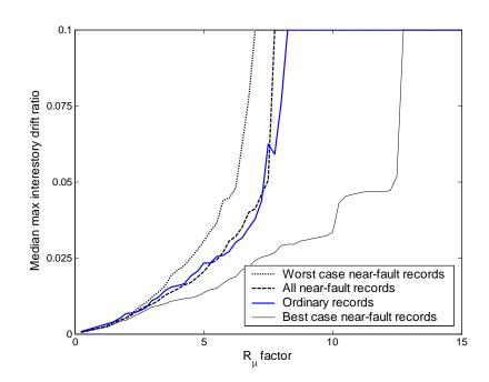
Figure 5.6. Median maximum interstory drift ratio versus normalized spectral acceleration  $(R_u)$  for the generic frame with 9 stories and a first-mode period of 0.9 seconds.
