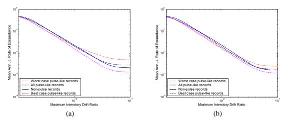
Figure 5.21. Drift hazard curves using the four considered record sets. (a) Curves computed using the scalar IM Sa(0.9s). (b) Curves computed using the vector IM consisting of Sa(0.9s)
