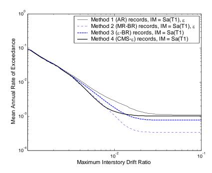
Figure F.6: Mean annual frequency of exceeding various levels of maximum interstory drift ratio, as computing using either the scalar intensity measure  $Sa(T_1)$  or the vector intensity measure  $Sa(T_1)$  and  $\varepsilon$ .
