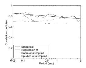
Figure 8.2. Correlation coefficients for perpendicular horizontal epsilons at the same period. Empirical results, the prediction from Equation 8.7, and the correlations implied from the ratios of standard deviations in Boore et al. (1997) and Spudich et al. (1999).
