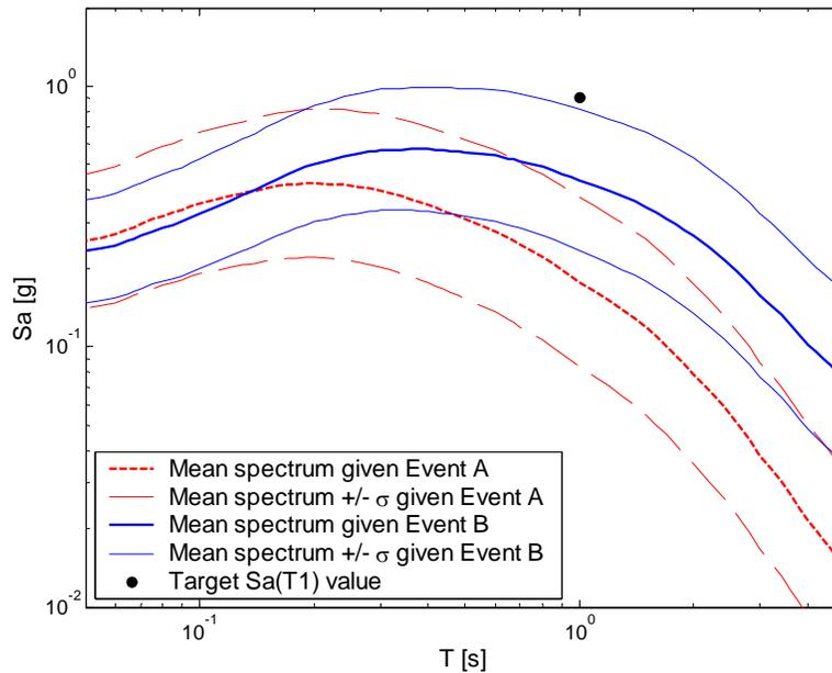
Figure E.4: Predicted mean spectra from the two possible events along with  $\pm$  one standard deviation. The target  $Sa(1s)$  value is also noted.
