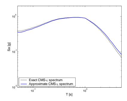
Figure E.6: Exact (using Equation E.2) and approximate (using Equation 6.1) CMS- $\varepsilon$  spectra for the given hypothetical site.
