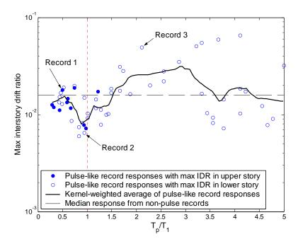
Figure 5.2. Maximum interstory drift ratio versus  $T_p/T_1$  for the generic frame with 9 stories and a first-mode period of 0.9 seconds, at an R<sub>µ</sub>-factor level of 4. Record 1: Morgan Hill, Anderson Dam (Magnitude = 6.2, Distance = 3km). Record 2: Kobe, KJMA (Magnitude = 6.9, Distance = 1km). Record 3: Superstition Hills, Parachute Test Site (Magnitude = 6.5, Distance = 1 km).
