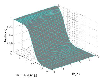
Figure 2.18. Probability of collapse predicted by fitting a joint normal distribution to collapse capacity as a function of  $\ln Sa(0.8s)$  and  $\varepsilon$ .
