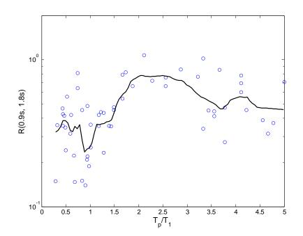
Figure 5.15.  $T_p$  versus  $R_{T1,T2}$  for the pulse-like ground motions, where  $T_1$ =0.9s and  $T_2$ =1.8s.
