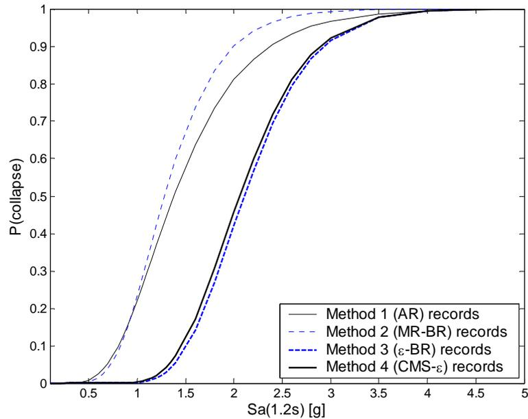
Figure F.10: Estimated probability of collapse vs.  $Sa(T_1)$  (i.e., the collapse “fragility curve”) using the four record-selection methods considered.
