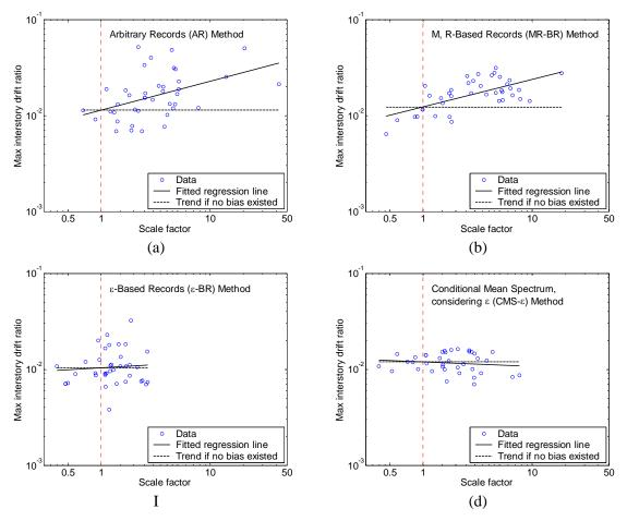
Figure 6.16: Maximum interstory drift ratio versus record scale factor for each of the four selection methods considered, at an Sa(0.8s) level of 0.6g. Regression fits based on scale factor are shown with solid lines. Dashed horizontal lines corresponding to the mean prediction at a scale factor of one are shown for comparison. (a) Records using the AR Method. (b) Records using the MR-BR Method. (c) Records using the  $\varepsilon$ -BR Method. (d) Records using the CMS- $\varepsilon$  Method.
