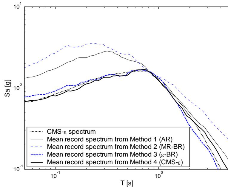
Figure 6.7: Conditional Mean Spectrum at  $Sa(0.8s)=1.6g$  (given  $\bar{M}=6.4$ ,  $\bar{R}=11.5$  km and  $\bar{\varepsilon}=2.1$ ) and the mean response spectra of record sets selected using each of the four proposed record selection methods.
