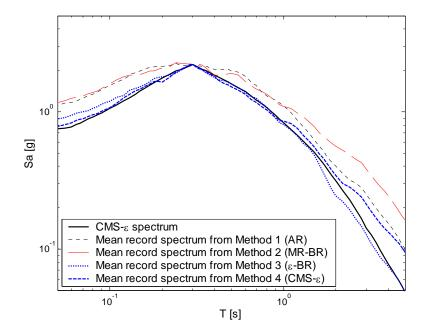
Figure F.1: Conditional Mean Spectra at Sa(0.3s)=2.2g (given  $\overline{M}=6.1$ ,  $\overline{R}=10.7$  km and  $\overline{\varepsilon}=2.1$ ) and the mean response spectra of record sets selected using each of the four proposed record selection methods.
