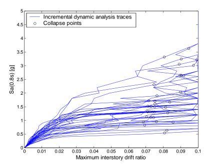
Figure D.1: Incremental dynamic analyses of the Van Nuys building, used to identify *Sa* values associated with collapse for each record.
