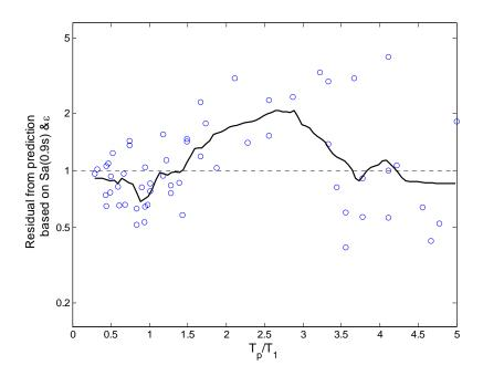
Figure 5.10. Residuals from response prediction based on  $Sa(T_1)$  and  $\varepsilon$  plotted versus  $T_p/T_1$  for the generic frame with 9 stories and a first-mode period of 0.9 seconds, at an  $R_{\mu}$  factor level of 4. No significant reduction in bias is seen, relative to Figure 5.9.
