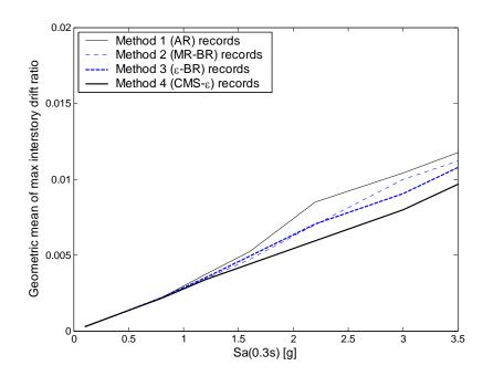
Figure F.2: The geometric mean of maximum interstory drift ratio vs.  $Sa(T_1)$  for the four record-selection methods considered.
