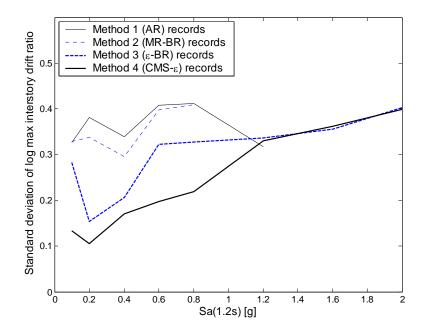
Figure F.9: The standard deviation of log maximum interstory drift ratio vs.  $Sa(T_1)$  for the four record-selection methods considered, at  $Sa(T_1)$  levels where less than 50% of records cause collapse.
