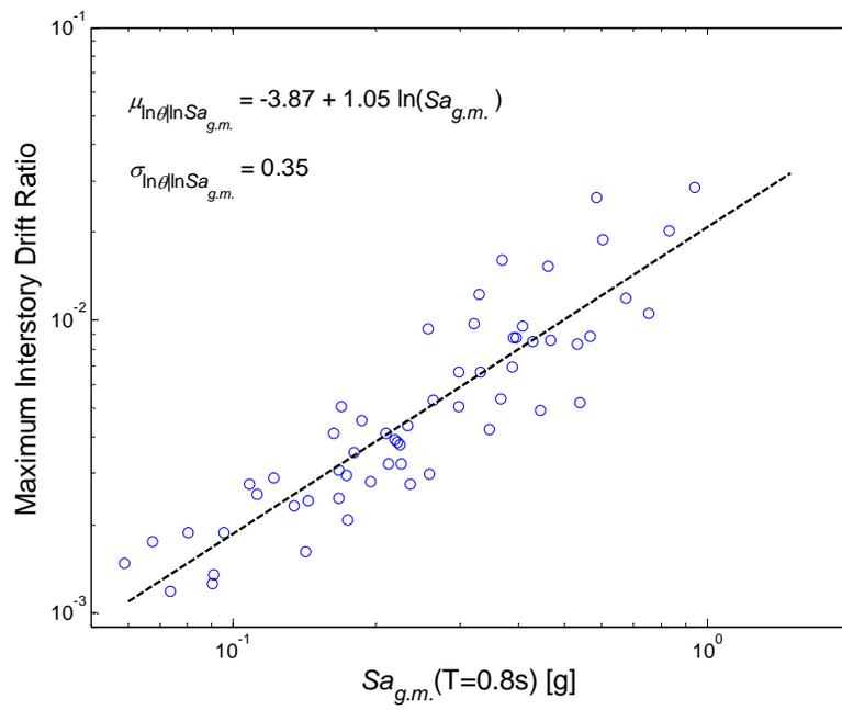
Figure 7.3. Prediction of the response of a single frame of a structure using (a) the spectral acceleration of the ground motion component used ( $Sa_{arb}$ ), and (b) the spectral acceleration of the average of both components ( $Sa_{g.m.}$ ).
