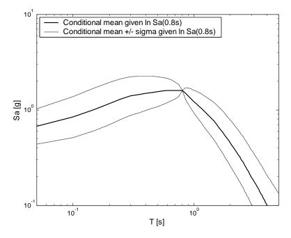
Figure 6.4: The distribution of spectral acceleration values, given Sa(0.8s) = 1.6g, and given  $\overline{M}$ ,  $\overline{R}$ ,  $\overline{\varepsilon}$  from PSHA disaggregation.
