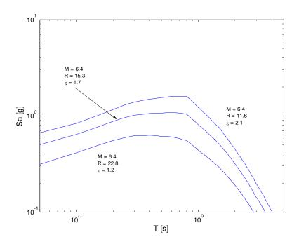
Figure 6.6: Mean values of the conditional response spectrum for a site in Van Nuys, California, given occurrence of Sa(0.8s) values exceeded with 2%, 10% and 50% probabilities in 50 years.
