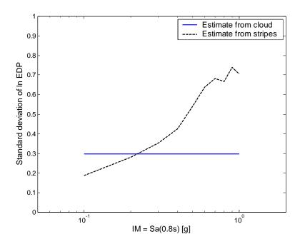
Figure 2.7. Standard deviation of  $\ln EDP | IM$  for non-collapse responses, estimated using the cloud and stripe methods. Only IM levels where less than 50% of records cause collapse are displayed because at levels with higher probability of collapse, the statistics estimated using only non-collapse responses are less meaningful.
