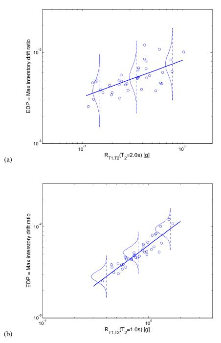
Figure 4.5: Comparison of the effectiveness of  $IM_2$  with two potential  $T_2$  values. (a) An  $IM_2$  choice with low efficiency; and (b) An  $IM_2$  with high efficiency
