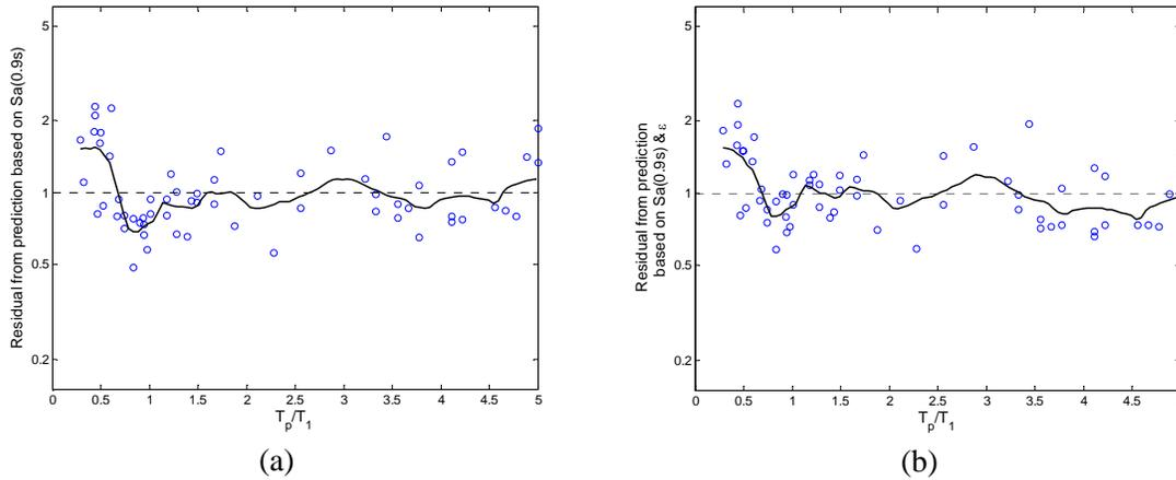
Figure 5.12. Residuals from response prediction based on (a)  $Sa(T_1)$  and (b)  $Sa(T_1)$  and  $\varepsilon$  plotted versus  $T_p/T_1$  for the generic frame with 9 stories and a first-mode period of 0.9 seconds, at an  $R_\mu$  level of 2. No significant reduction in bias is seen when  $\varepsilon$  is incorporated in the intensity measure.
