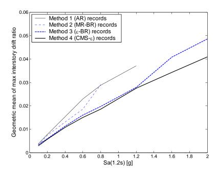
Figure F.8: The geometric mean of maximum interstory drift ratio vs.  $Sa(T_1)$  for the four record-selection methods considered.
