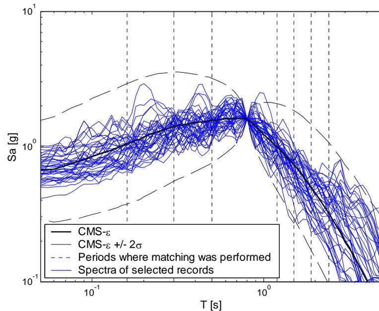
Figure 6.5: The Conditional Mean Spectrum considering  $\varepsilon$ , the CMS- $\varepsilon$   $\pm$  two  $\sigma$ , and response spectra of records selected based on their match with this spectral shape. All spectra are conditioned upon  $Sa(0.8s)=1.6g$ .
