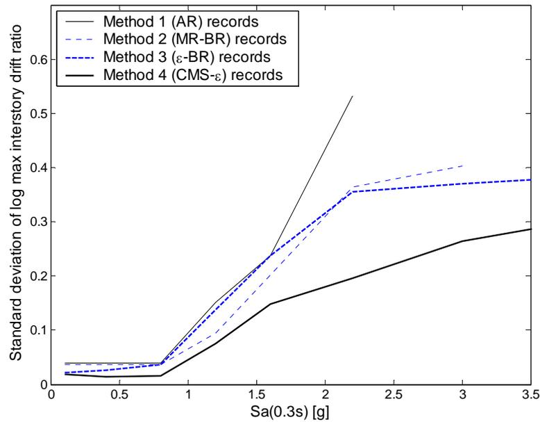
Figure F.3: The standard deviation of log maximum interstory drift ratio vs.  $Sa(T_1)$  for the four record-selection methods considered, at  $Sa(T_1)$  levels where less than 50% of records cause collapse.
