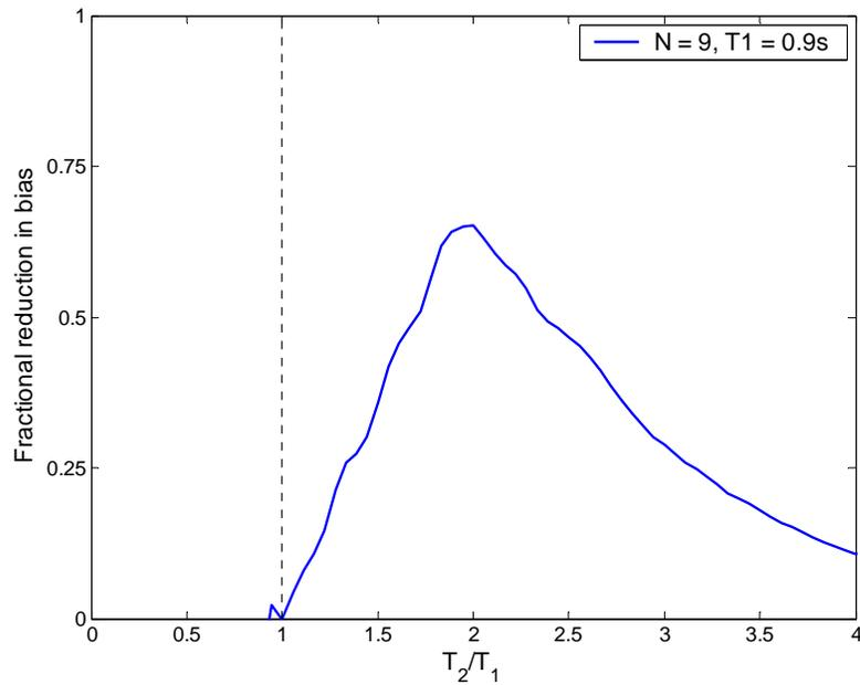
Figure 5.17. Percent reduction in the proposed bias statistic versus the  $T_2$  value used in  $R_{T_1, T_2}$ . Results are shown for the  $N=9$ ,  $T_1 = 0.9\text{s}$  structure with an  $R_\mu$  factor of 4.
