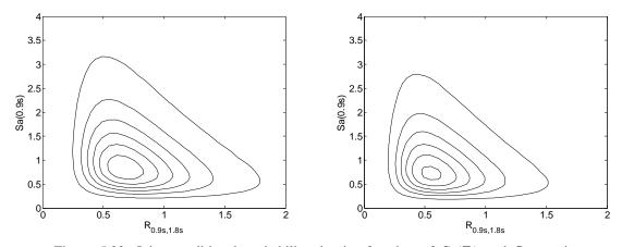
Figure 5.22. Joint conditional probability density function of  $Sa(T_1)$  and  $R_{T_1,T_2}$ , given a Magnitude 7 event at a distance of 5km, with the near-fault parameters X=0.5 and  $\theta$ =5%.  $T_1$ =0.9s and  $T_2$ =1.8s, in the fault-normal direction. (a) With near-fault effects considered. (b) Without near-fault effects considered.
