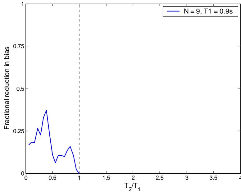
Figure 5.20. Percent reduction in the proposed bias statistic versus the  $T_2$  value used in  $R_{T_1, T_2}$ . Results are shown for the  $N=9$ ,  $T_1 = 0.9\text{s}$  structure with an  $R_\mu$  factor of 2.
