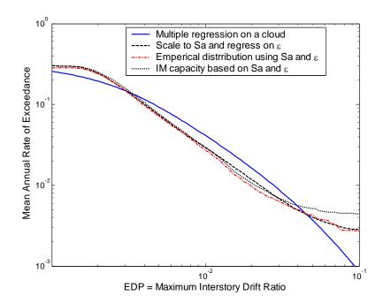
Figure 2.20. Comparison of drift hazard results using a vector-valued intensity measures consisting of  $Sa(T_1)$  and  $\varepsilon$ .
