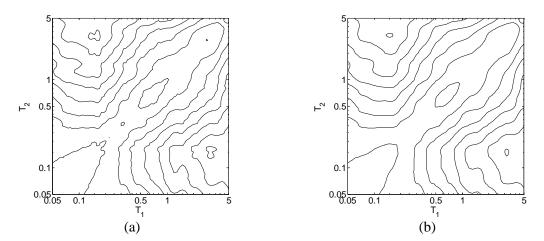
Figure 8.1. Effect of smoothing on the empirical correlation matrix for horizontal epsilons in perpendicular directions at two periods (T1 and T2). (a) Before smoothing. (b) After smoothing.
