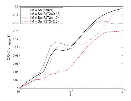
Figure 4.17: Coefficient of variation vs. *EDP* level for three candidate vector *Ims* and the scalar *IM*.
