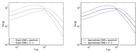
Figure E.7: (a) Exact conditional mean and standard deviation of the response spectrum, given Sa(1s)=0.9g. (using Equations E.2 and E.3). (b) Approximate conditional mean and standard deviation of the response spectrum, given Sa(1s)=0.9g. (using Equations 6.1 and 6.2).
