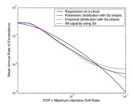
Figure 2.9. Comparison of drift hazard results for the example structure using the four estimation methods described above.
