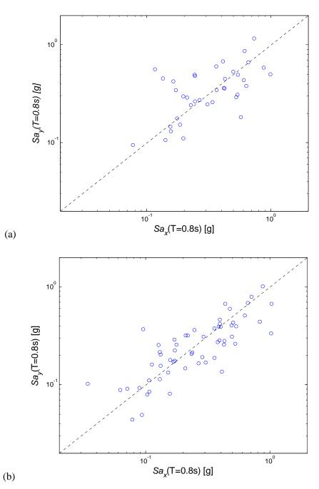
Figure 7.5. Samples of  $(\ln Sa_x, \ln Sa_y)$  pairs from (a) a set of ground motions with magnitude  $\approx$  6.5 and distance  $\approx$  8km, and (b) a set of ground motions with a wider range of magnitudes and distances, used to perform the structural analyses displayed in Figure 7.3.
