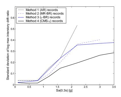
Figure F.3: The standard deviation of log maximum interstory drift ratio vs.  $Sa(T_1)$  for the four record-selection methods considered, at  $Sa(T_1)$  levels where less than 50% of records cause collapse.
