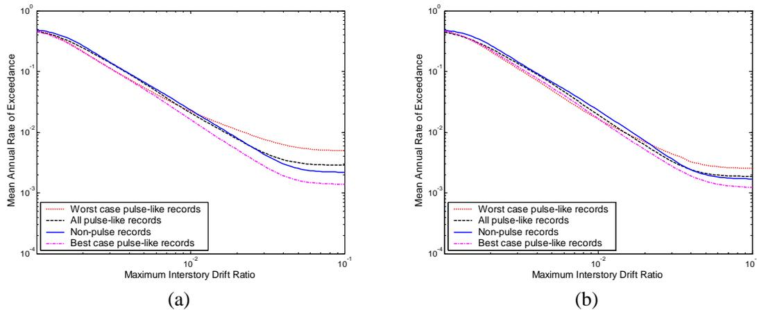
Figure 5.21. Drift hazard curves using the four considered record sets. (a) Curves computed using the scalar IM  $Sa(0.9s)$ . (b) Curves computed using the vector IM consisting of  $Sa(0.9s)$
