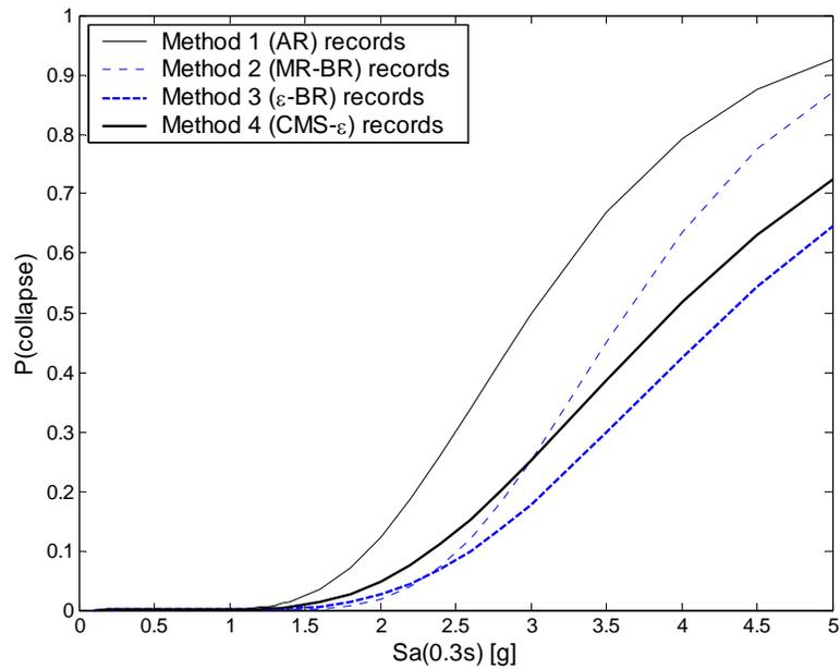
Figure F.4: Estimated probability of collapse vs.  $Sa(T_1)$  (i.e., the collapse “fragility curve”) using the four record-selection methods considered.
