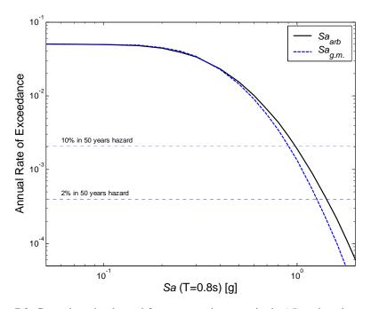
Figure 7.2. Ground motion hazard from a recurring magnitude 6.5 earthquake at a distance of 8 kilometers, for  $Sa_{arb}$  and  $Sa_{g.m.}$  at a period of 0.8 seconds with 5% damping
