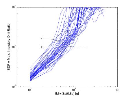
Figure 2.5. Incremental dynamic analysis curves, and an estimated (lognormal) CDF of  $IM_{cap}$  given maximum interstory drift ratio = 0.01.
