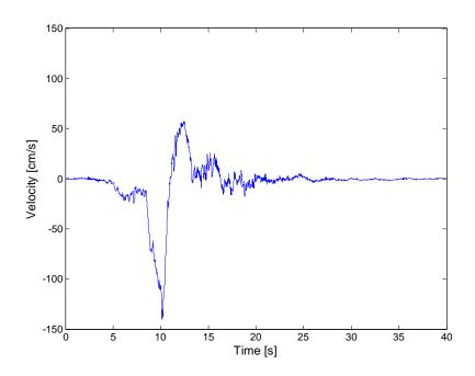
Figure 5.1. The velocity time history of the fault-normal horizontal ground motion recorded at Lucern during the 1992 Landers earthquake. A "pulse" is clearly present.
