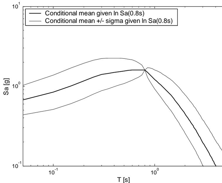
Figure 6.4: The distribution of spectral acceleration values, given  $Sa(0.8s) = 1.6g$ , and given  $\bar{M}$ ,  $\bar{R}$ ,  $\bar{\varepsilon}$  from PSHA disaggregation.
