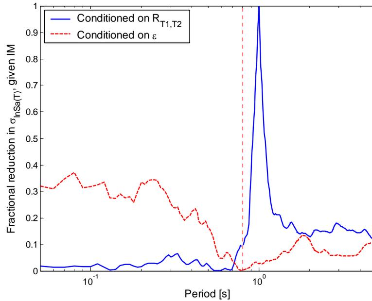
Figure 4.19: Fractional reduction in standard deviation of  $S_a(T)$  given  $S_a(T_1)$  after conditioning on  $R_{T_1, T_2}$  or  $\varepsilon$ .  $T_1=0.8\text{s}$ ,  $T_2=1.0\text{s}$ .
