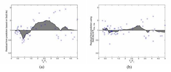
Figure 5.16. Area under the kernel-weighted average line, to be used as a proxy for the total bias as a function of  $T_p$ . Results are for the generic frame with 9 stories and a first-mode period of 0.9 seconds,  $T_2$ =1.8s, and  $R_{\mu}$ =4. (a) Bias when using  $Sa(T_1)$  as the IM. (b) Bias when using  $Sa(T_1)$  and  $R_{T1,T2}$ , as the IM. The total area is reduced by 65% when the vector IM is adopted.
