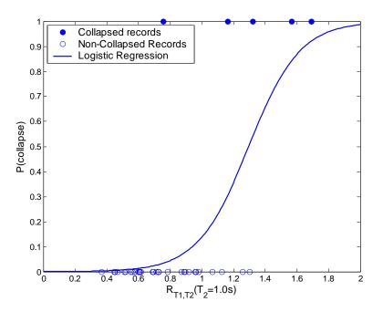
Figure 4.3: An example of prediction of the probability of collapse using logistic regression applied to binary collapse/non-collapse results ( $S_a(T_1) = 0.9g$ ).
