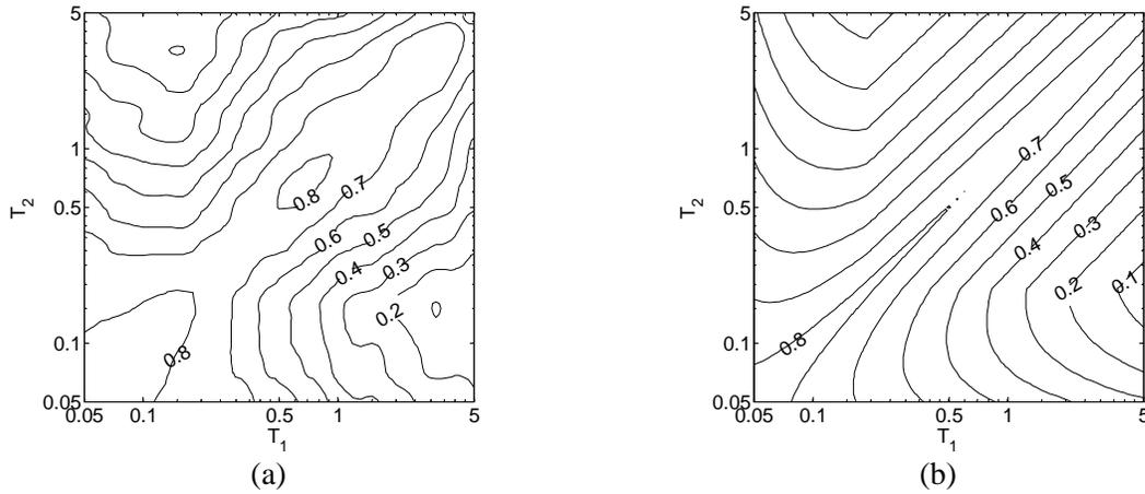
Figure 8.6. Correlation contours for horizontal epsilons in perpendicular directions at two periods ( $T_1$  and  $T_2$ ). (a) Smoothed empirical results. (b) The prediction from Equation 8.11.
