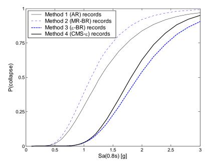
Figure 6.11: Estimated probability of collapse vs.  $Sa(T_1)$  (i.e., the collapse "fragility curve") using the four record-selection methods considered.
