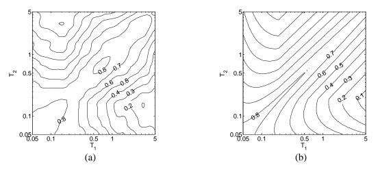
Figure 8.6. Correlation contours for horizontal epsilons in perpendicular directions at two periods ( $T_1$  and  $T_2$ ). (a) Smoothed empirical results. (b) The prediction from Equation 8.11.
