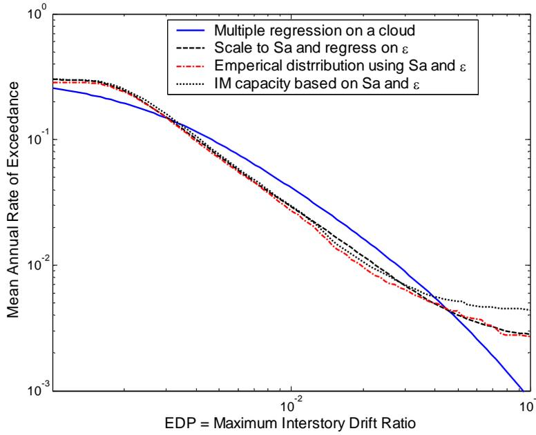
Figure 2.20. Comparison of drift hazard results using a vector-valued intensity measures consisting of  $Sa(T_1)$  and  $\varepsilon$ .
