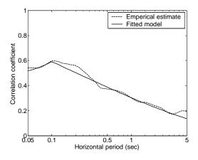
Figure 8.8. Correlation coefficient between vertical epsilons and horizontal epsilons when the period in the vertical direction is 0.1 seconds.
