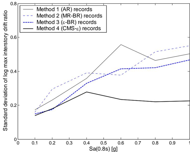
Figure 6.10: The standard deviation of log maximum interstory drift ratio for records that do not cause collapse, plotted versus  $Sa(T_1)$  for the four record-selection methods considered.
