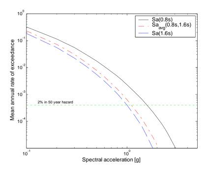
Figure 6.17: Hazard curves for  $\ln Sa(0.8s)$ ,  $\ln Sa(1.6s)$ , and  $\ln Sa_{avg}(0.8s, 1.6s)$  at the Van Nuys site.
