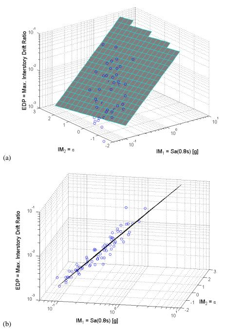
Figure 2.10. (a) The mean fit from a cloud of data, predicted using multiple linear regression with Sa(0.8s) and  $\varepsilon$  as predictors. (b) The same mean from a different viewpoint, to emphasize that the prediction is a plane.
