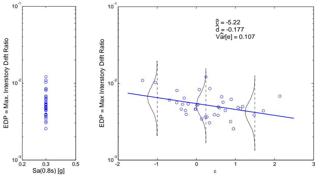
Figure 2.13. Prediction of response given no collapse, at  $Sa(0.8s) = 0.3g$ , with the distribution of the residuals superimposed over the data.
