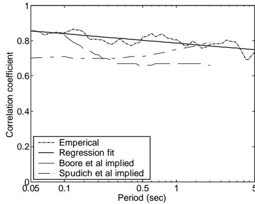
Figure 8.2. Correlation coefficients for perpendicular horizontal epsilons at the same period. Empirical results, the prediction from Equation 8.7, and the correlations implied from the ratios of standard deviations in Boore et al. (1997) and Spudich et al. (1999).
