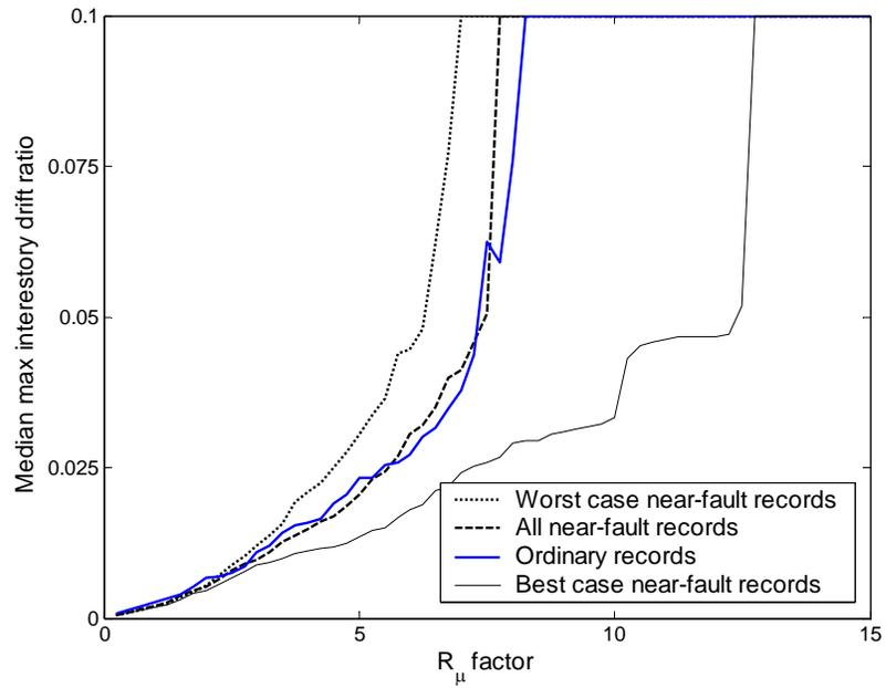
Figure 5.6. Median maximum interstory drift ratio versus normalized spectral acceleration ( $R_\mu$ ) for the generic frame with 9 stories and a first-mode period of 0.9 seconds.
