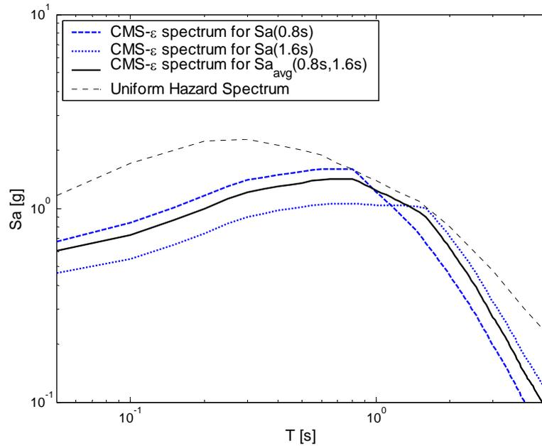
Figure 6.18: CMS- $\epsilon$  spectra for  $\ln Sa(0.8s)$ ,  $\ln Sa(1.6s)$ , and  $\ln Sa_{avg}(0.8s,1.6s)$  at the 2% in 50 year hazard level, and the 2% in 50 year uniform hazard spectrum.
