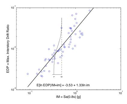
Figure 2.1. A cloud of EDP|IM data, the conditional mean value from linear regression, and the CCDF of EDP given Sa(0.8s) = 0.5g.
