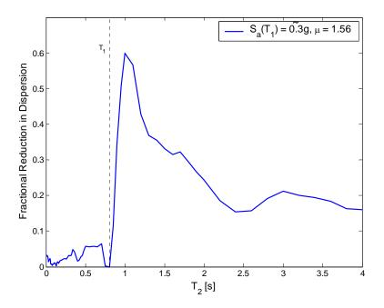
Figure 4.6: Fractional reduction in dispersion vs.  $T_2$  for  $T_2$  between 0 and 4 seconds for  $S_a(T_1)=0.3$ g.
