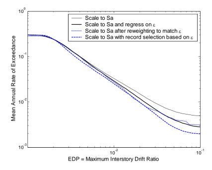
Figure 2.21. Comparison of drift hazard results using the vector-IM based regression procedure of Section 2.5.2, the record selection procedure of Section 2.6.1 and the reweighting procedure of Section 2.6.2. The scalar intensity measure used is Sa(0.8s), and the vector is Sa(0.8s) and  $\varepsilon$ .
