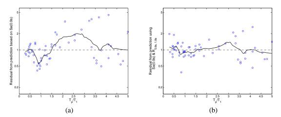
Figure 5.14. Residuals from response prediction based on (a)  $Sa(T_1)$  only, and (b) both  $Sa(T_1)$  and  $R_{T_1,T_2}$ , plotted versus  $T_p/T_1$  for the generic frame with 9 stories and a first-mode period of 0.9 seconds, at an  $R_{\mu}$  factor level of 4.  $T_2$ =1.8s for this plot.
