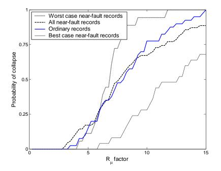
Figure 5.7. Counted probabilities of collapse versus normalized spectral acceleration for the frame with 9 stories and a first-mode period of 0.9 seconds.
