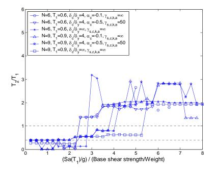
Figure 4.11: The optimal  $T_2$ , normalized by first-mode period ( $T_1$ ) for a set of six- and ninestory structures with moderate contribution from second-mode response.
