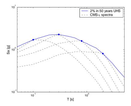
Figure 6.15: 2% in 50 years uniform hazard spectrum at the Van Nuys site, along with several Conditional Mean Spectra, considering  $\varepsilon$  (CMS- $\varepsilon$ ), conditioned on *Sa*(*T*) at four different values of *T* (0.1, 0.3, 0.8 and 2 seconds).
