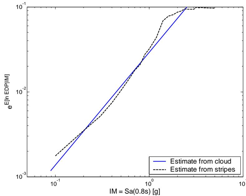
Figure 2.6. Mean values of  $EDP|IM$  for non-collapsing records, estimated using the cloud and stripe methods. For the stripe method, the values between stripes are determined using linear interpolation.
