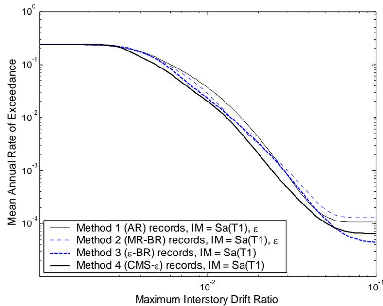
Figure F.12: Mean annual frequency of exceeding various levels of maximum interstory drift ratio, as computing using either the scalar intensity measure  $Sa(T_1)$  or the vector intensity measure  $Sa(T_1)$  and  $\epsilon$ .
