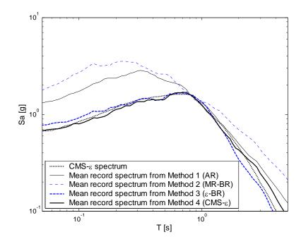
Figure 6.7: Conditional Mean Spectrum at Sa(0.8s)=1.6g (given  $\overline{M} = 6.4$ ,  $\overline{R} = 11.5$  km and  $\overline{\varepsilon} = 2.1$ ) and the mean response spectra of record sets selected using each of the four proposed record selection methods.
