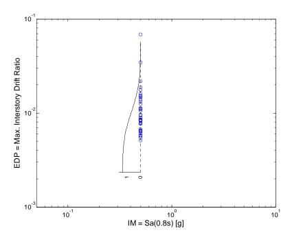
Figure 2.2. A stripe of data and its estimated complementary cumulative distribution function from a fitted parametric distribution.
