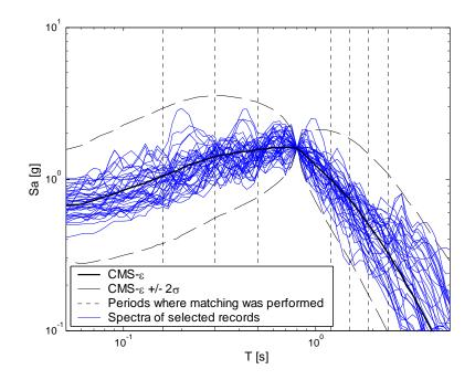
Figure 6.5: The Conditional Mean Spectrum considering  $\varepsilon$ , the CMS- $\varepsilon$  +/- two  $\sigma$ , and response spectra of records selected based on their match with this spectral shape. All spectra are conditioned upon Sa(0.8s)=1.6g.
