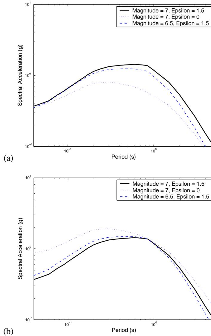
Figure 3.5. (a) Expected response spectra for three scenario events; (b) expected response spectra for three scenario events, scaled to have the same  $S_a(0.8s)$  value.
