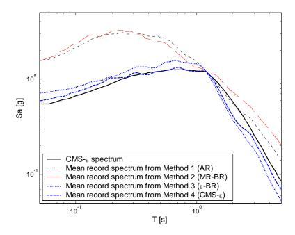
Figure F.7: Conditional Mean Spectrum at Sa(1.2s)=1.2g (given  $\overline{M} = 6.6$ ,  $\overline{R} = 15.8$  km and  $\overline{\varepsilon} = 2.1$ ) and the mean response spectra of record sets selected using each of the four proposed record selection methods.
