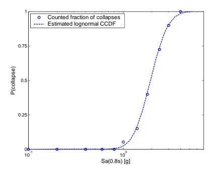
Figure D.4: Empirical probability of collapse and a lognormal distribution fitted using generalized linear regression with a Probit link function.
