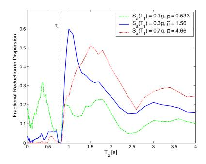
Figure 4.7: Fractional reduction in dispersion vs.  $T_2$  for three levels of  $S_a(T_1)$ .
