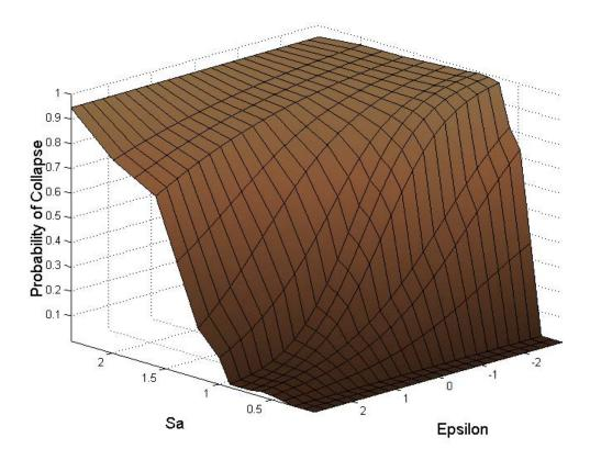
Figure 3.2. Prediction of the probability of collapse as a function of both  $S_a(T_1)$  and  $\varepsilon$ .
