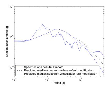
Figure C.1. The response spectrum of the Lucerne recording from the 1992 Landers earthquake, along with predicted median spectra from ground motion prediction models with and without near-fault effects accounted for.
