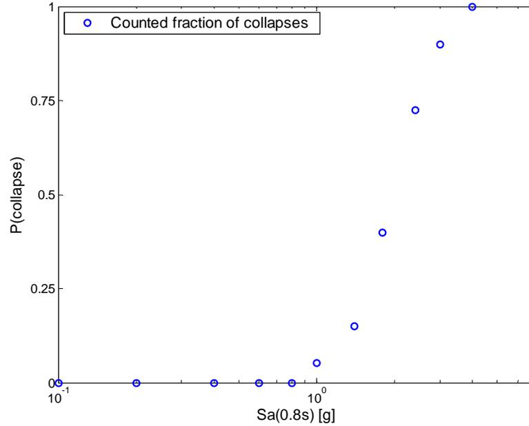
Figure D.3: Empirical probability of collapse for a set of  $Sa$  values, obtained from records selected to match target epsilon values at each  $Sa$  level.
