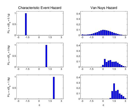
Figure 3.6. Disaggregation of PSHA results. The conditional distribution of  $\varepsilon$  given  $S_a(0.8s)=x$  is shown for both fault models at three different hazard spectral acceleration levels associated with three different mean annual frequencies of exceedance.
