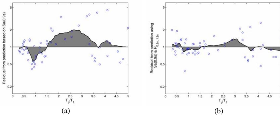
Figure 5.16. Area under the kernel-weighted average line, to be used as a proxy for the total bias as a function of  $T_p$ . Results are for the generic frame with 9 stories and a first-mode period of 0.9 seconds,  $T_2=1.8s$ , and  $R_\mu=4$ . (a) Bias when using  $Sa(T_1)$  as the IM. (b) Bias when using  $Sa(T_1)$  and  $R_{T_1, T_2}$ , as the IM. The total area is reduced by 65% when the vector IM is adopted.
