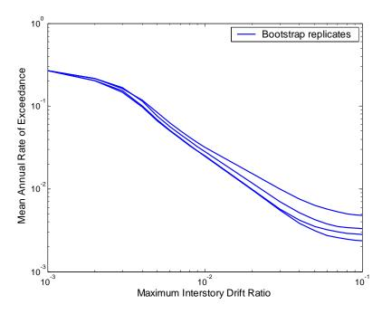
Figure 4.15: Bootstrap replicates of the vector IM drift hazard curve
