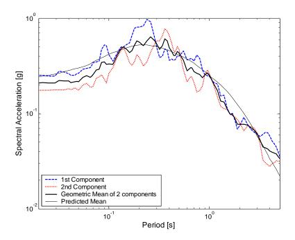
Figure 7.1. Response spectra from the magnitude 6.2 Chalfant Valley earthquake recorded at Bishop LADWP, 9.2 km from the fault rupture. Response spectra for the two horizontal components of the ground motion, the geometric mean of the response spectra, and the predicted mean for the given magnitude and distance using the prediction of Abrahamson and Silva (1997).
