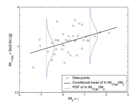
Figure 2.17. Sa(0.8s),  $\varepsilon$  pairs corresponding to occurrence of 0.1 maximum interstory drift ratio.
