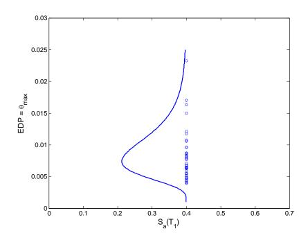
Figure 4.2: Structural response results from dynamic analysis using forty records scaled to  $S_a(T_1) = 0.4g$ , and a superimposed lognormal probability density function, generated using the method of moments.
