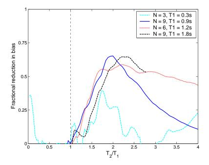
Figure 5.18. Percent reduction in the proposed bias statistic versus the  $T_2$  value used in  $R_{T1,T2}$ . Results are shown for all four structures, each with an  $R_{\mu}$  factor of 4.
