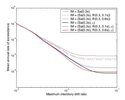
Figure 4.18: Maximum interstory drift hazard curves computed using a scalar *IM*, twoparameter *Ims*, and three-parameter *Ims*. Results shown are for the 3-story structure with  $T_1=0.3$ s,  $\delta_c/\delta_y=4$ ,  $\alpha_c=-0.1$  and  $\gamma_{s,c,k,a}=\infty$  (see Table 3.1).
