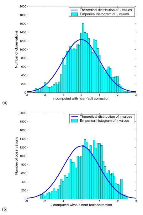
Figure C.2. Histograms of  $\varepsilon$  values computed for the 70 near-fault ground motions at periods from 0.6 seconds to 5.0 seconds, both with (a) and without (b) modification to account for near-fault effects.
