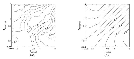
Figure 8.7. Correlation contours of vertical epsilons with horizontal epsilons at two periods  $(T_1 \text{ and } T_2)$ . (a) Smoothed empirical results. (b) The prediction from Equation 8.12.
