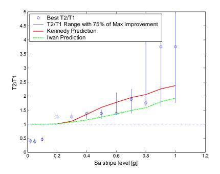
Figure 4.8: The optimum second period  $T_2$ , versus the level of  $S_a(T_1)$ .
