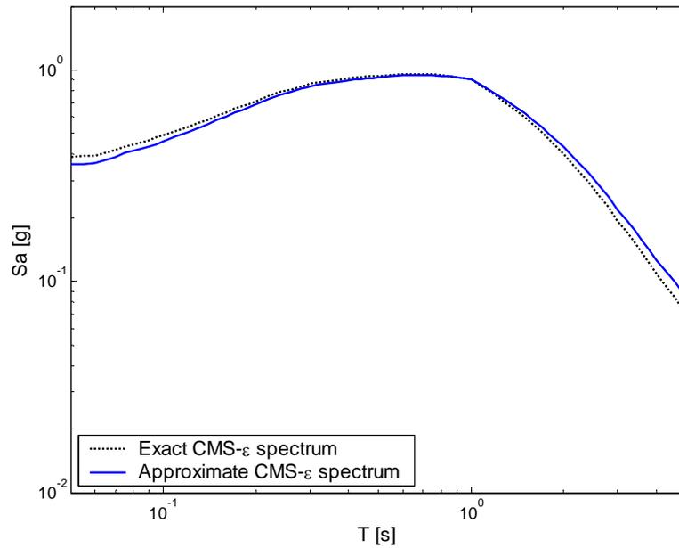
Figure E.6: Exact (using Equation E.2) and approximate (using Equation 6.1) CMS- $\epsilon$  spectra for the given hypothetical site.
