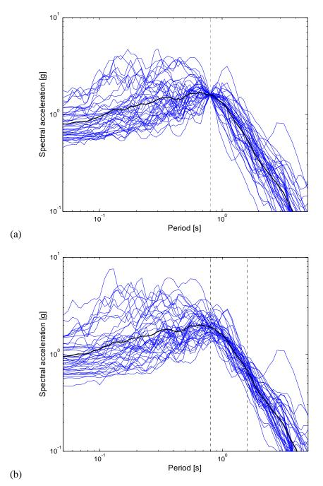
Figure 6.20: Records scaled to target 2% in 50 year IM levels. (a) Records scaled to  $\ln Sa(0.8s)$ . (b) Records scaled to  $\ln Sa_{avg}(0.8s, 1.6s)$ .
