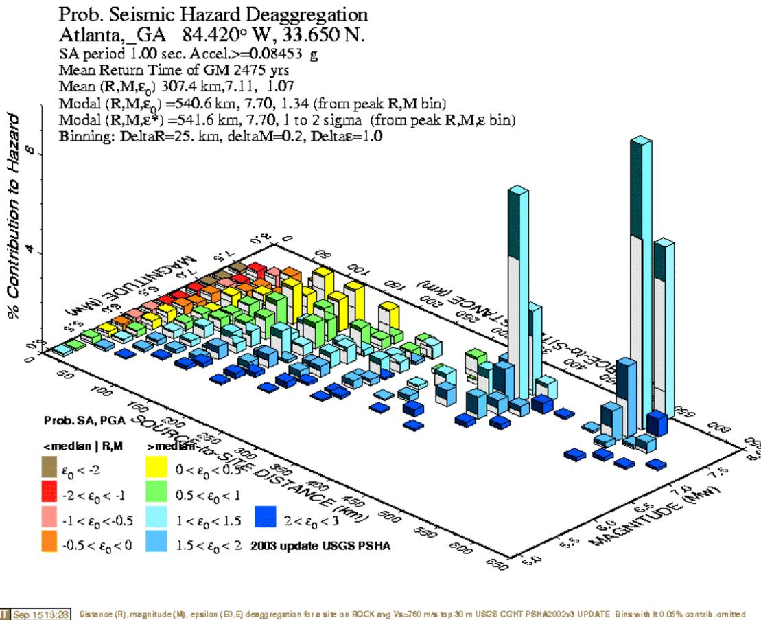
Figure E.8: Disaggregation for  $Sa(1.0s)$  at the 2% in 50 year hazard level for Atlanta, Georgia (USGS 2002).
