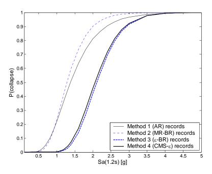
Figure F.10: Estimated probability of collapse vs.  $Sa(T_1)$  (i.e., the collapse "fragility curve") using the four record-selection methods considered.
