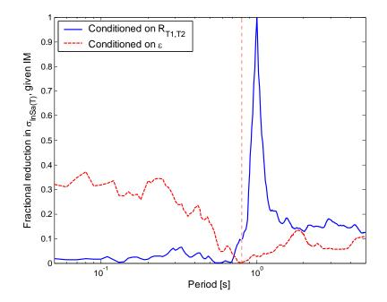
Figure 4.19: Fractional reduction in standard deviation of Sa(T) given  $Sa(T_1)$  after conditioning on  $R_{T_1,T_2}$  or  $\varepsilon$ .  $T_1$ =0.8s,  $T_2$ =1.0s.
