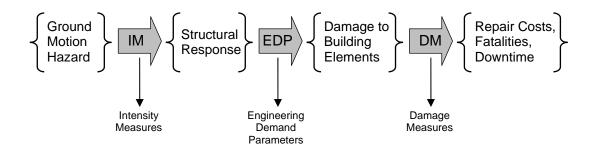
Figure 1.1: Schematic illustration of the Performance-Based Earthquake Engineering model and the pinch points IM, EDP and DM.
