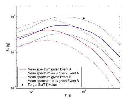
Figure E.4: Predicted mean spectra from the two possible events along with +/- one standard deviation. The target *Sa*(1s) value is also noted.
