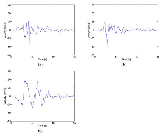
Figure 5.4. Velocity time histories of the three example pulse-like ground motions, after scaling each so that Sa(0.9s)=0.5g. (a) Record 1: Morgan Hill, Anderson Dam ( $T_p = 0.4s$ , Magnitude = 6.2, Distance = 3km). (b) Record 2: Kobe, KJMA ( $T_p = 0.9s$ , Magnitude = 6.9, Distance = 1km). (c) Record 3: Superstition Hills, Parachute Test Site ( $T_p = 2.9s$ , Magnitude = 6.5, Distance = 1 km).
