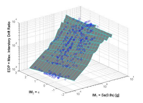
Figure 2.14. Conditional mean fit of non-collapse responses from stripes of data, predicted by scaling records to Sa(0.8s) and using repeated regressions with  $\varepsilon$  as the predictor.
