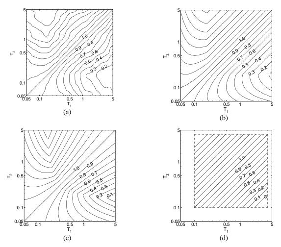
Figure 8.4. Correlation contours for horizontal epsilons in the same direction at two periods (T1 and T2). (a) Smoothed empirical results. (b) The prediction from Equation 8.9. (c) The prediction from Abrahamson et al. (2003). (d) The prediction from Inoue and Cornell (1990).
