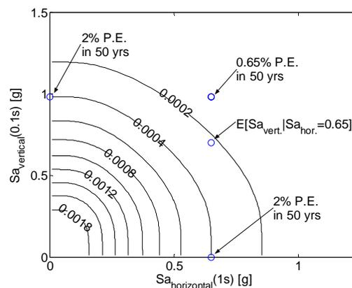
Figure 8.10. Contours of vector-valued probabilistic seismic hazard analysis. The contours denote the mean annual rate of exceeding *both* the  $Sa_{\text{vertical}}$  *and* the  $Sa_{\text{horizontal}}$  values.
