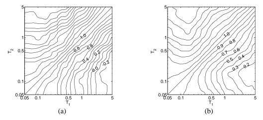
Figure C.3. Empirical correlation contours for horizontal spectral acceleration values in the same direction at two periods ( $T_1$  and  $T_2$ ) for (a) pulse-like and (b) ordinary ground motions.
