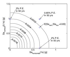
Figure 8.10. Contours of vector-valued probabilistic seismic hazard analysis. The contours denote the mean annual rate of exceeding *both* the Sa<sub>vertical</sub> *and* the Sa<sub>horizontal</sub> values.
