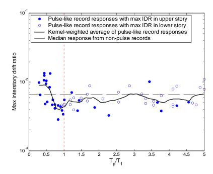
Figure 5.5. Maximum interstory drift ratio versus  $T_p/T_1$  for the generic frame with 9 stories and a first-mode period of 0.9 seconds, at an  $R_\mu$  level of 2.
