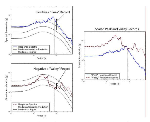
Figure 3.3. Scaling a negative  $\varepsilon$  record and a positive  $\varepsilon$  record to the same  $S_a(T_1)$ : an illustration of the peak and valley effect. In this case,  $T_1 = 0.8$  seconds.
