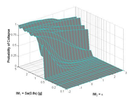
Figure 2.12. Probability of collapse fit from stripes of data, predicted by scaling to Sa(0.8s) and using repeated logistic regressions with  $\varepsilon$  as the predictor.
