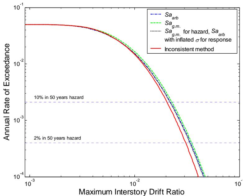
Figure 7.4. Drift hazard as computed using the three methods proposed above and the inconsistent method.
