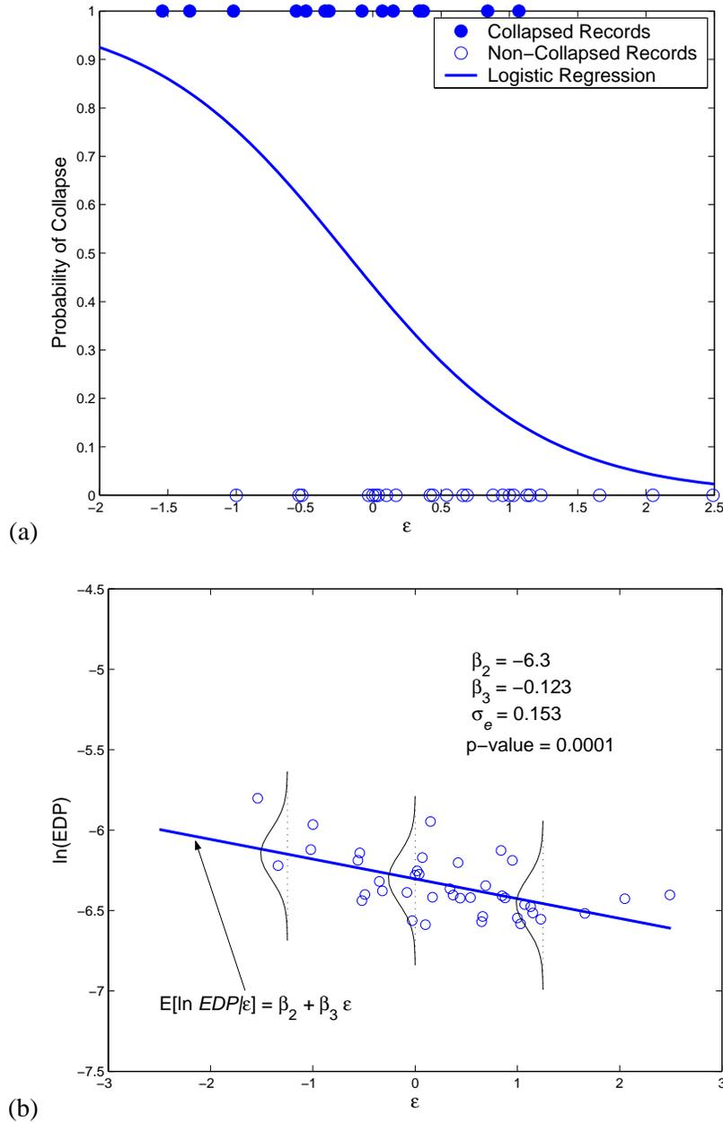
Figure 3.1. Analysis of data at a fixed value of  $S_a$ , (a) Prediction of the probability of collapse using logistic regression applied to binary collapse/non-collapse results; and (b) prediction of response given no collapse, with the distribution of the residuals superimposed over the data.
