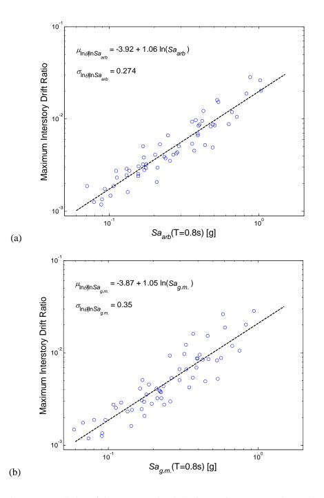
Figure 7.3. Prediction of the response of a single frame of a structure using (a) the spectral acceleration of the ground motion component used ( $Sa_{arb}$ ), and (b) the spectral acceleration of the average of both components ( $Sa_{g.m.}$ ).
