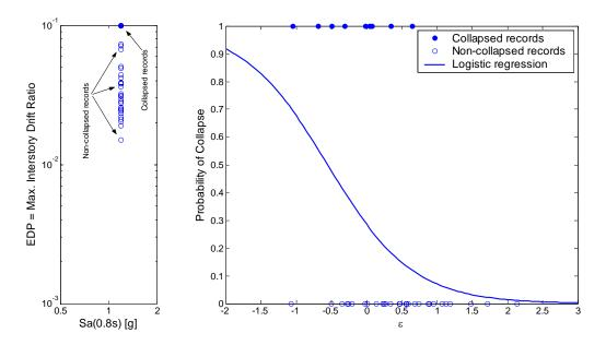
Figure 2.11. Prediction of the probability of collapse using logistic regression applied to binary collapse/non-collapse results at Sa(0.8s) = 1.2g.
