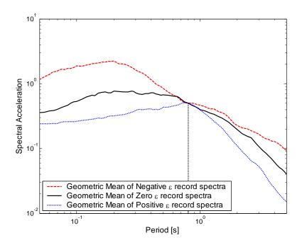
Figure 6.2: The geometric mean of response spectra for negative- $\varepsilon$ , zero- $\varepsilon$  and positive- $\varepsilon$  record sets, after each record's spectrum has been scaled to Sa(0.8s)=0.5g.
