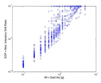
Figure 2.3. Multiple stripes of data used to re-estimate distributions at varying *IM* levels. Note that records that cause maximum interstory drift ratios of larger than 0.1 are displayed with interstory drift ratios of 0.1.
