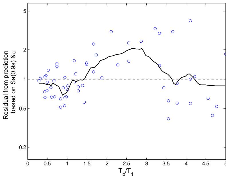
Figure 5.10. Residuals from response prediction based on  $Sa(T_1)$  and  $\varepsilon$  plotted versus  $T_p/T_1$  for the generic frame with 9 stories and a first-mode period of 0.9 seconds, at an  $R_u$  factor level of 4. No significant reduction in bias is seen, relative to Figure 5.9.
