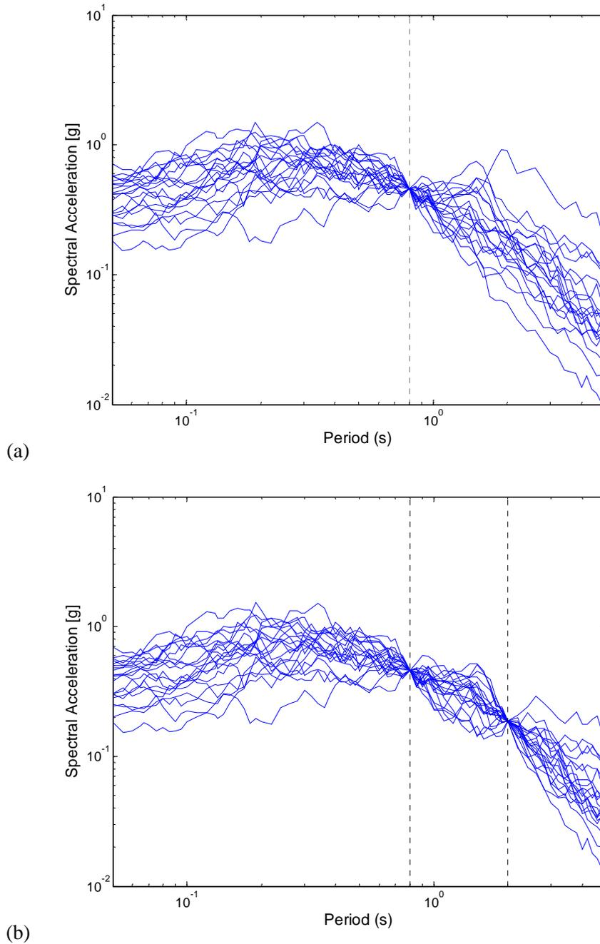
Figure 2.19. (a) Response spectra of records scaled to match spectral acceleration at a 0.8s. (b) Response spectra of records scaled to match spectral acceleration at 0.8s and processed to match spectral acceleration at 2.0s.
