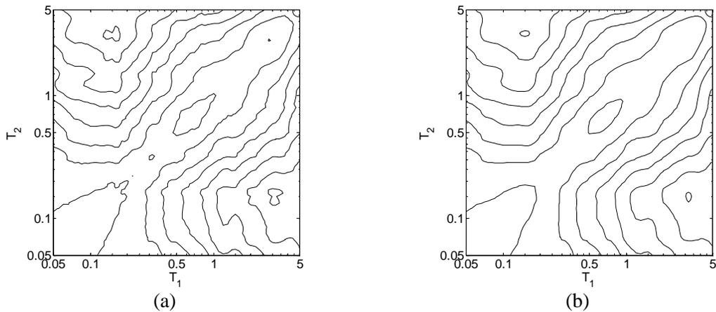
Figure 8.1. Effect of smoothing on the empirical correlation matrix for horizontal epsilons in perpendicular directions at two periods ( $T_1$  and  $T_2$ ). (a) Before smoothing. (b) After smoothing.
