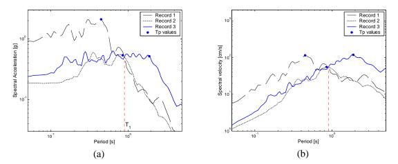
Figure 5.3. (a) Acceleration, and (b) velocity spectra of the three highlighted records from Figure 5.2, after scaling each record so that Sa(0.9s) = 0.5g.
