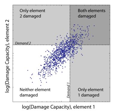
Figure 2: An illustration of the joint distribution of damage capacities for two elements. Points represent Monte Carlo simulations of the damage capacities for the two elements, and shaded regions indicate areas where the structural demand has exceeded the damage capacity for one or both elements.
