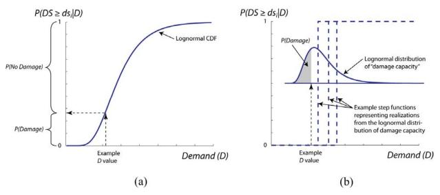
Figure 1: Two equivalent representations of an element fragility. (a) A lognormal CDF specifying the probability of collapse. (b) A step function specifying the probability of collapse, with the location of the step described by a lognormal distribution.
