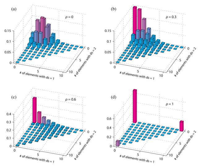
Figure 4: Probability of observing n damaged components out of 10, when there are two potential damage states and  $P(DS \ge 1) = 0.3$  and  $P(DS \ge 2) = 0.1$ , for four correlation coefficient values. (a)  $\rho = 0$  (uncorrelated fragilities). (b)  $\rho = 0.3$ . (c)  $\rho = 0.6$ . (d)  $\rho = 1$  (perfectly correlated fragilities).
