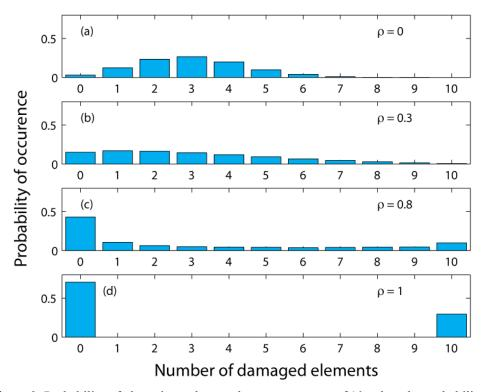
Figure 3: Probability of observing n damaged components out of 10, when the probability of damage of a single component is equal to 0.3, for four correlation coefficient values. (a)  $\rho$ =0 (uncorrelated fragilities). (b)  $\rho$ =0.3. (c)  $\rho$ =0.8. (d)  $\rho$ =1 (perfectly correlated fragilities).
