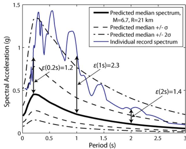
Figure 5. Response spectra from the example Castaic Old Ridge Route ground motion, used to illustrate calculation of  $\epsilon$  values at three periods. Note that the  $\pm \sigma$  bands are not symmetric around the median because they are  $\pm \sigma$  values of  $\ln Sa$ , rather than (non-log)  $Sa$ .
