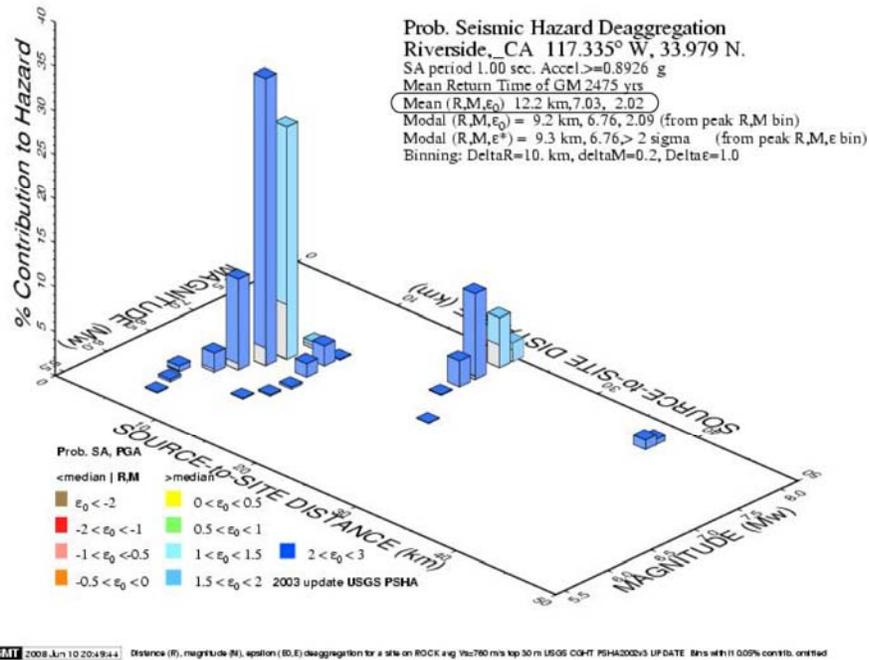
Figure 2. PSHA deaggregation for Riverside, given  $Sa(1s) > 0.89g$ . (Figure from USGS Custom Mapping and Analysis Tools, <http://earthquake.usgs.gov/research/hazmaps/interactive/>, 2008. Emphasis on mean deaggregation values added by the author.)
