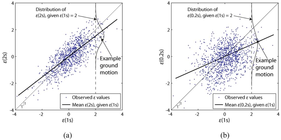
Figure 6. Scatter plots of  $\epsilon$  values from a large suite of ground motions. The points associated with the ground motion in Figure 5 are highlighted. (a)  $\epsilon(1s)$  versus  $\epsilon(2s)$ . (b)  $\epsilon(1s)$  versus  $\epsilon(0.2s)$ .
