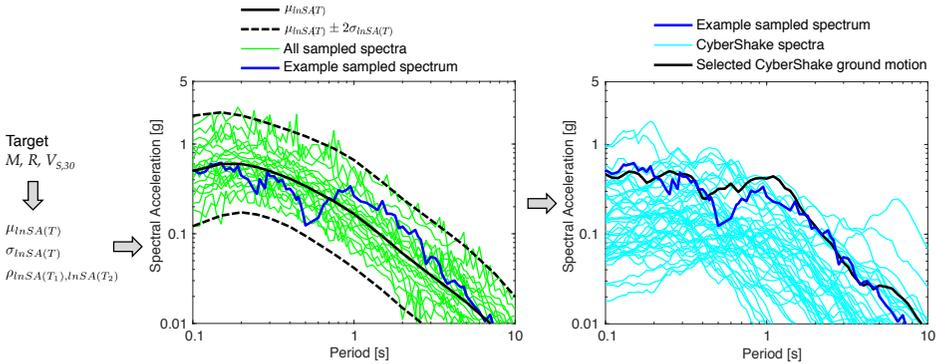
**Figure 5.** Schematic illustration of the ground-motion selection process. We first specify a target scenario and compute the means, standard deviations and correlations of  $lnSA$  (left); we then sample response spectra from the resulting distribution (middle); finally, we compare each sampled response spectrum to the CyberShake spectra and select the closest match (right).
