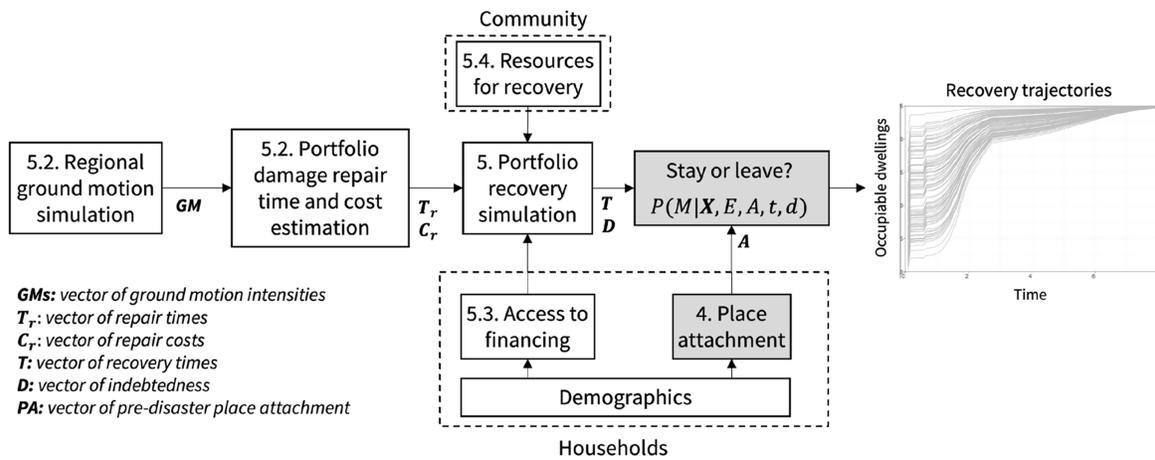
**Fig. 1.** Schematic representation of a housing recovery simulation model. The numbers in each box indicate the sequence in which the models are discussed. The shaded boxes indicate the contributions of this study.
