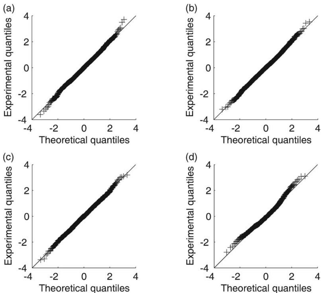
**Figure 1.** The normal  $Q-Q$  plots of the normalized intraevent residuals at four different periods. (a)  $T = 0.5$  sec (1560 samples); (b)  $T = 1.0$  sec (1548 samples); (c)  $T = 2.0$  sec (1498 samples); and (d)  $T = 10.0$  sec (507 samples).
