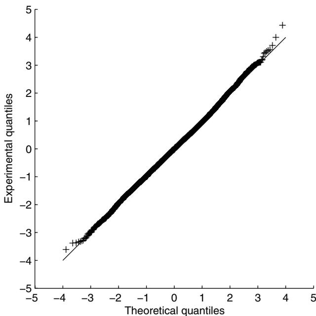
**Figure 3.** The normal  $Q-Q$  plot of the pooled set of normalized intraevent residuals.
