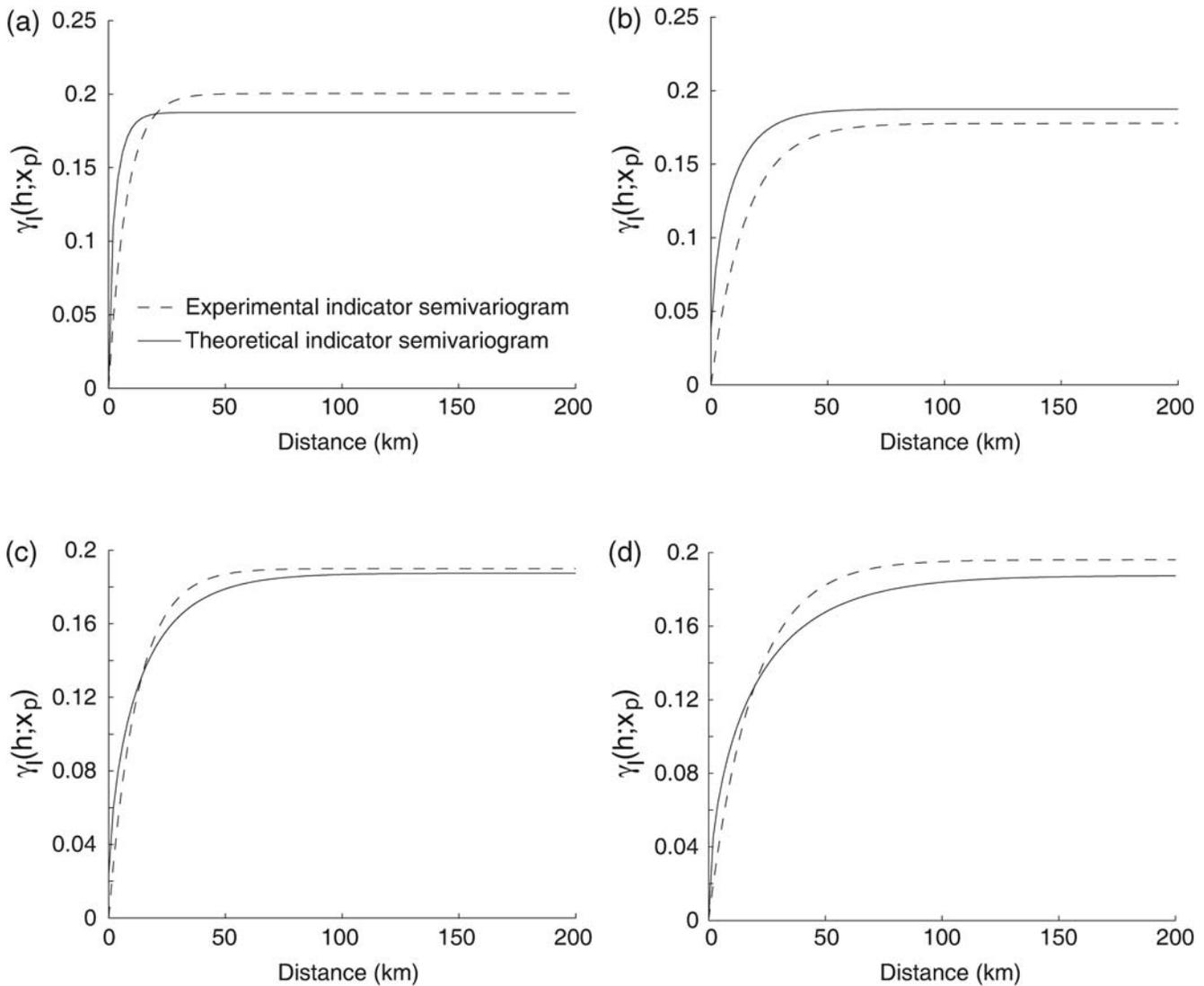
**Figure 6.** Theoretical and empirical semivariograms for the 0.25 quantile of the residuals. (a) results for the residuals computed at 0.5 sec from the Northridge data; (b) results for the residuals computed at 0.5 sec from the Chi-Chi data; (c) results for the residuals computed at 1 sec from the Chi-Chi earthquake data; and (d) results for the residuals computed at 5 sec from the Chi-Chi data.
