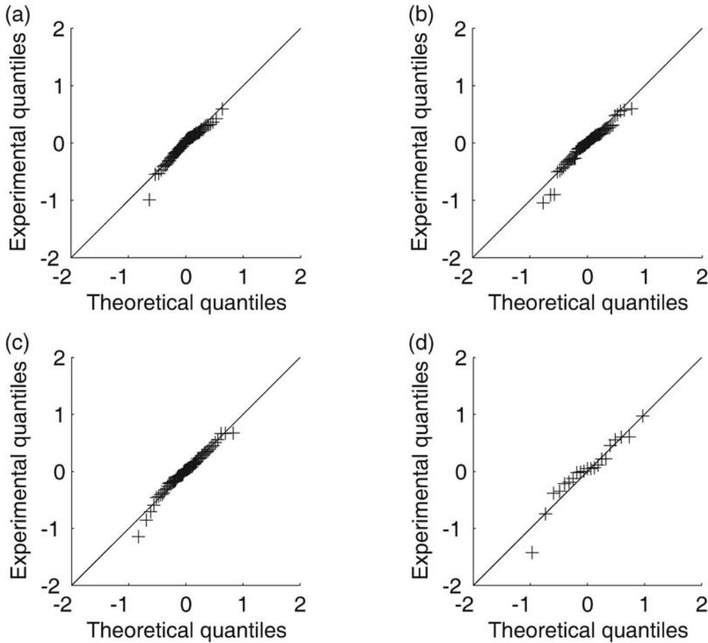
**Figure 4.** The normal  $Q-Q$  plots of interevent residuals at four different periods. (a)  $T = 0.5$  sec (64 samples); (b)  $T = 1.0$  sec (64 samples); (c)  $T = 2.0$  sec (62 samples); and (d)  $T = 10.0$  sec (21 samples).
