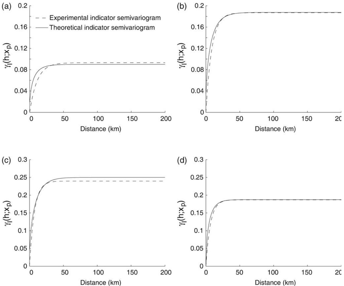
**Figure 5.** Theoretical and empirical semivariograms for residuals computed at 2 sec. (a) Results for the 0.1 quantile of the residuals from the Chi-Chi data; (b) results for the 0.25 quantile of the residuals from the Chi-Chi data; (c) results for the 0.5 quantile of the residuals based from the Chi-Chi data; and (d) results for the 0.25 quantile of the residuals from the Northridge data.
