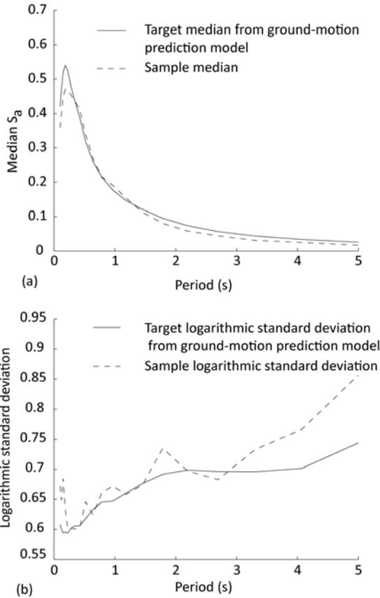
Figure 5 Rock sites: (a) Comparison of the target and the sample medians, and (b) Comparison of the target and the sample logarithmic standard deviations.
