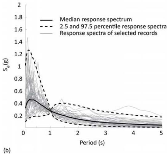
Figure 7 Case 1: Conditional response spectra of the scaled selected ground motions for soil sites (a) Log-Log plot, and (b) Linear plot.
