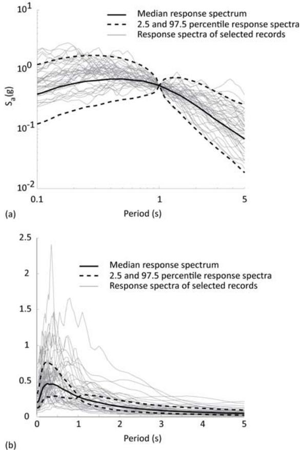
Figure 9 Case 2: Conditional response spectra of the scaled selected ground motions for soil sites (a) Log-Log plot, and (b) Linear plot.
