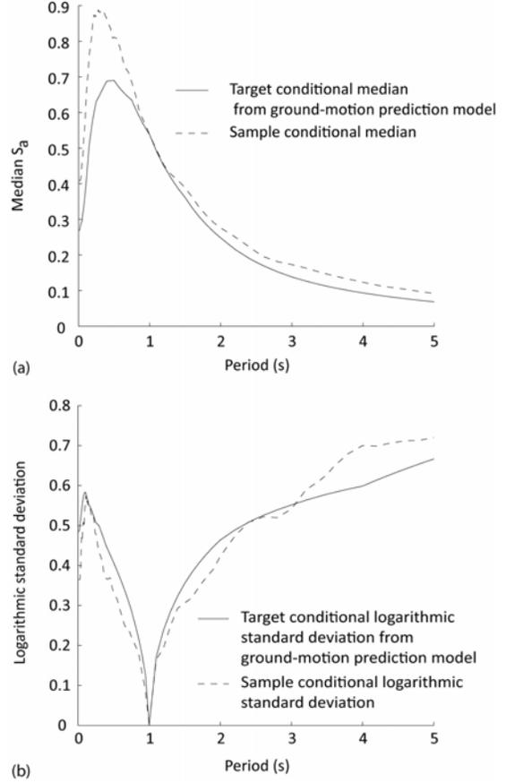
Figure 10 Case 2: (a) Comparison of the conditional target and sample medians, and (b) Comparison of the conditional target and sample logarithmic standard deviations.
