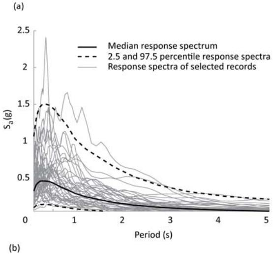
Figure 1 Response spectra of the selected ground motions for soil sites (a) Log-Log plot, and (b) Linear plot.
