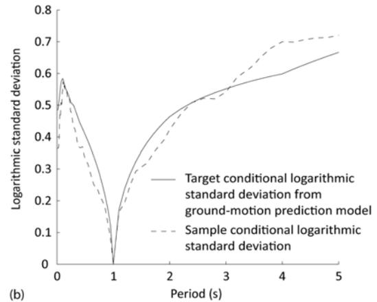
Figure 8 Case 1: (a) Comparison of the conditional target and sample medians, and (b) Comparison of the conditional target and sample logarithmic standard deviations.
