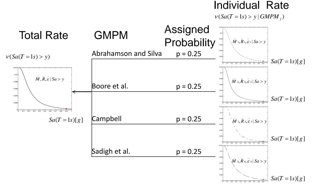
•Here we consider ways to incorporate multiple GMPMs, using refinements to disaggregation and conditional mean spectrum (CMS).
