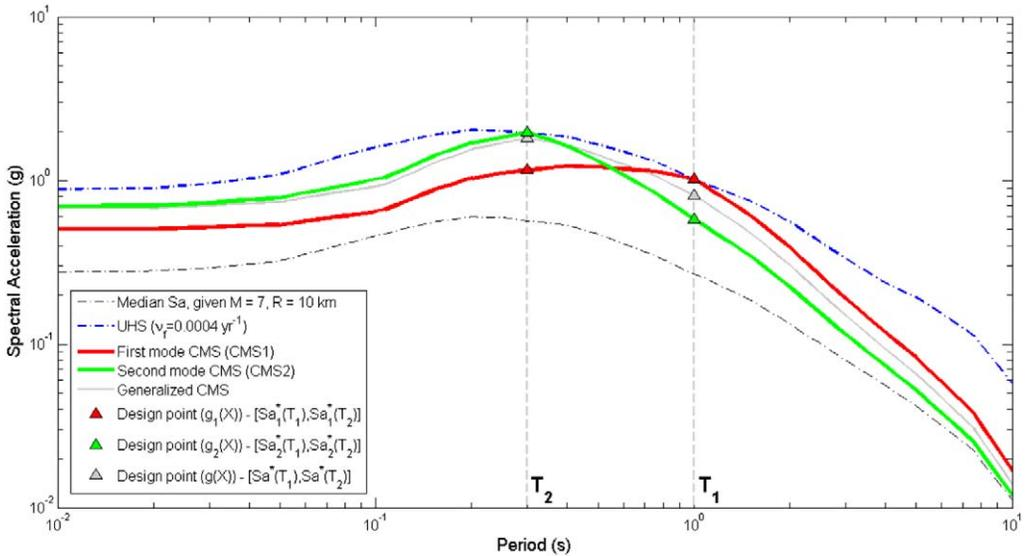
**Figure 5.** Response spectra associated with the FORM calculations for the two-period *EDP* example.
