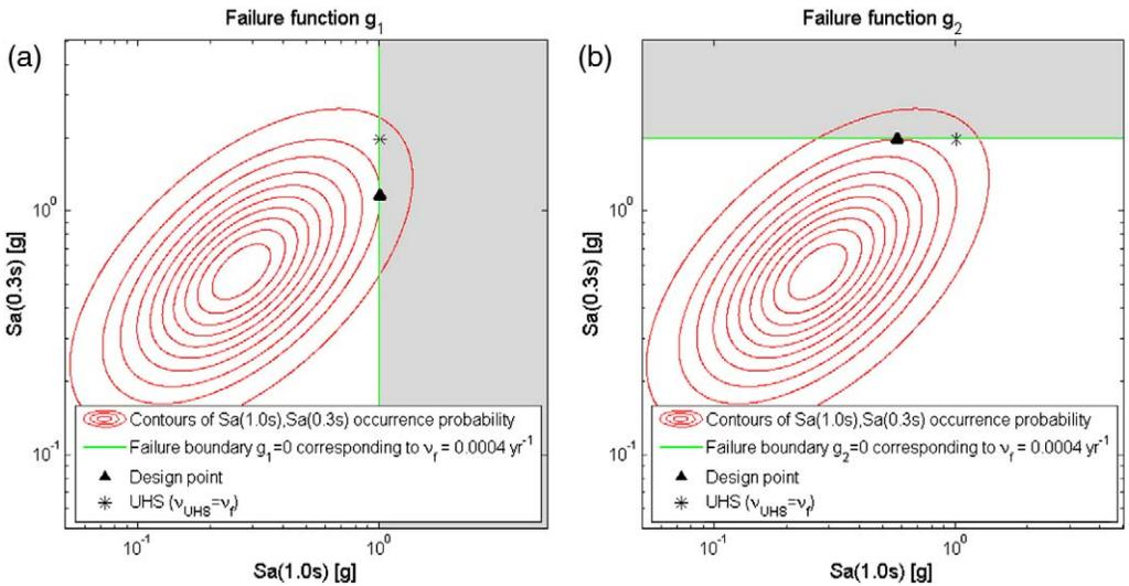
**Figure 4.** Limit state functions and design points for (a) the first-mode limit-state function of Equation 14 and (b) the second-mode limit state function of Equation 16.
