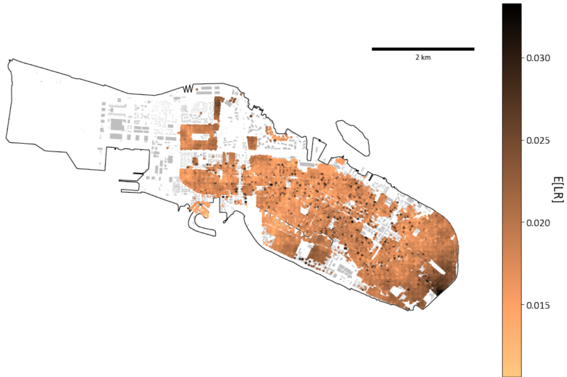
Fig. 7. Map of expected annual loss ratio at each residential building location. The darker color corresponds to the higher E[LR] values, and lighter colors signify a lower expected loss. Non-colored locations are areas without residential buildings.
