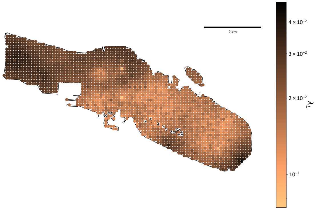
Fig. 4. Annual rate of liquefaction occurrence, as computed using Eq. 5. The lightest color refers to the lowest rates and therefore lower probability of liquefaction, and darker signifies higher rates or more hazardous areas.
