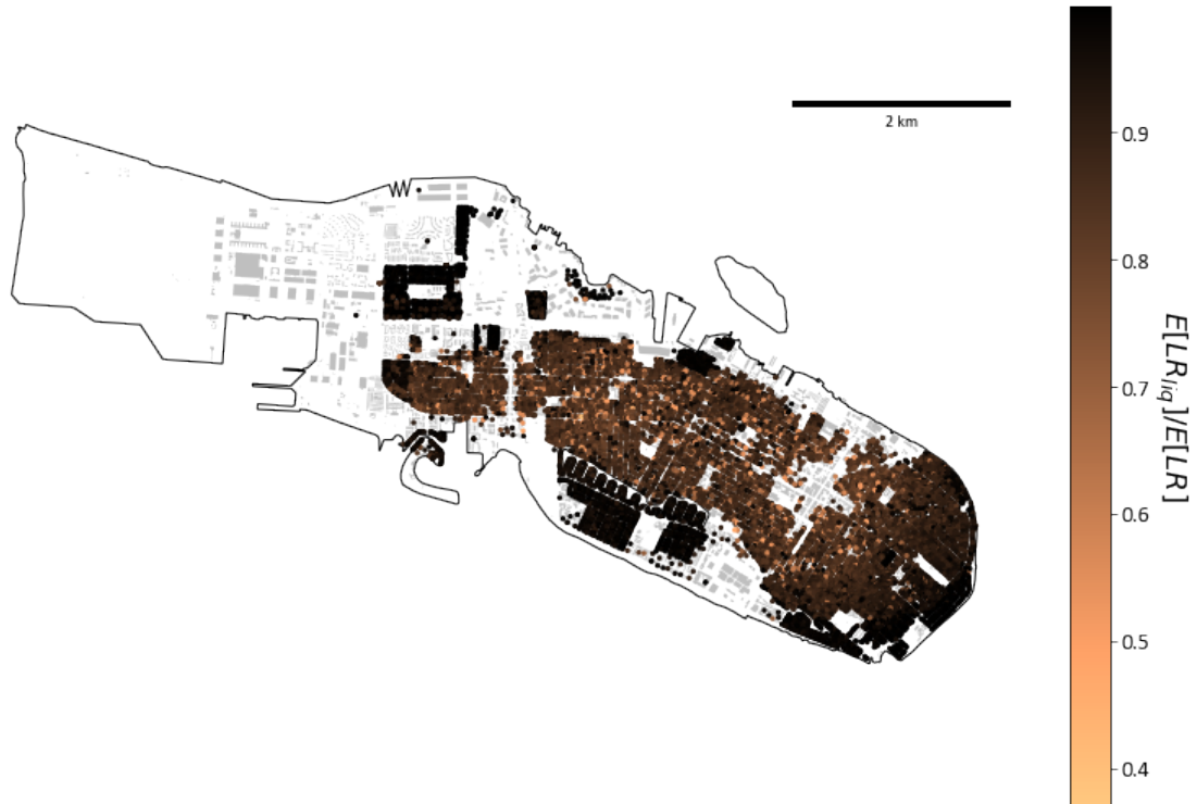
Fig. 8. Map of the expected fraction of building loss ratio attributable to liquefaction hazard.
