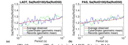
Figure 3.  $Sa_{RotD100}(T)/Sa_{RotD50}(T)$  for (a) site LADT, (b) site PAS, compared against the average observed ratio from NGA-West2
