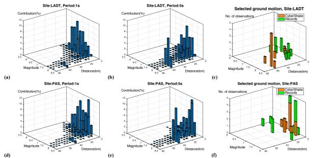
Figure 1. Deaggregation for site LADT at (a) 1s, (b) 5s, (c) magnitude and distance of selected ground motions for site LADT, deaggregation for site PAS at (d) 1s, (e) 5s, (f) magnitude and distance of selected ground motions for site PAS
