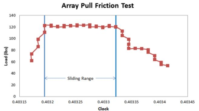
**Figure 9:** Sample test plot from example friction pull test of a PV array
