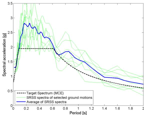
**Figure 8:** Target MCE for *Intensity Level 2*, site classes A-D, horizontal SRSS spectra of the scaled ground motions representing this analysis case, and the average of the selected and scaled spectra.
