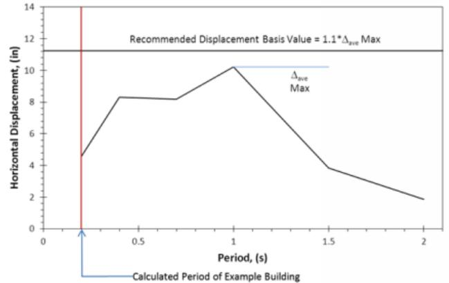
**Figure 13:** Calculated response vs. recommended seismic clearance
