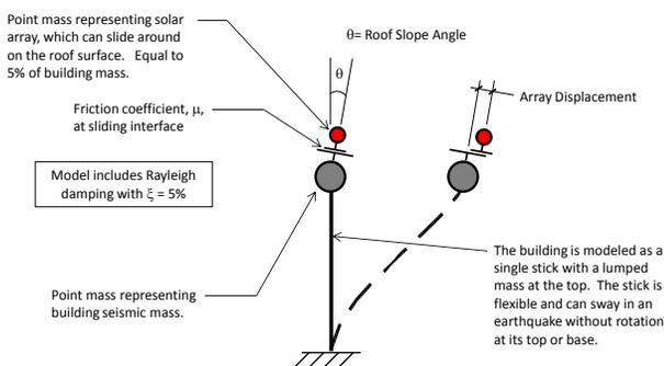
**Figure 10:** Schematic Representation of Analysis Model
