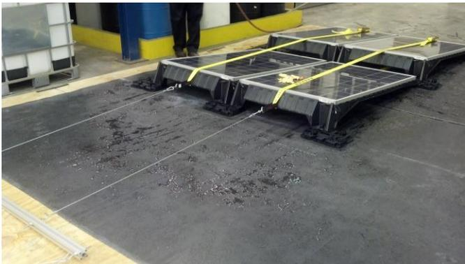
**Figure 5:** Example of full scale array pull testing.
