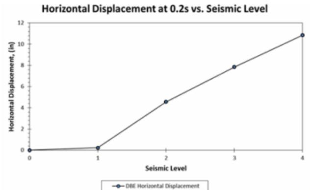
**Figure 14:** Displacement Occurrence Threshold Corresponding to *Seismic Intensity Level*
