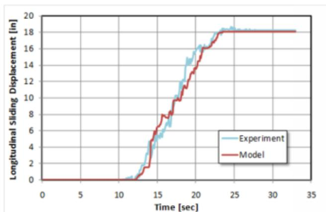
**Figure 20:** Comparison of shake test results with analysis.
