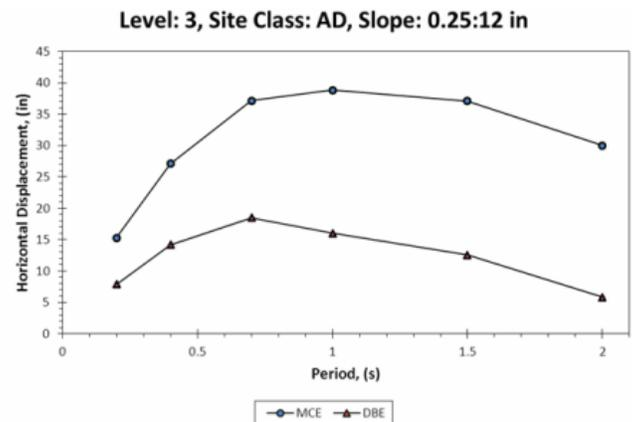
**Figure 18:** Horizontal displacement comparison at MCE/DBE levels. Site Class A through D with slope at 1/4": 12
