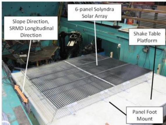
**Figure 19:** Photograph of assembled array on shake table platform.
